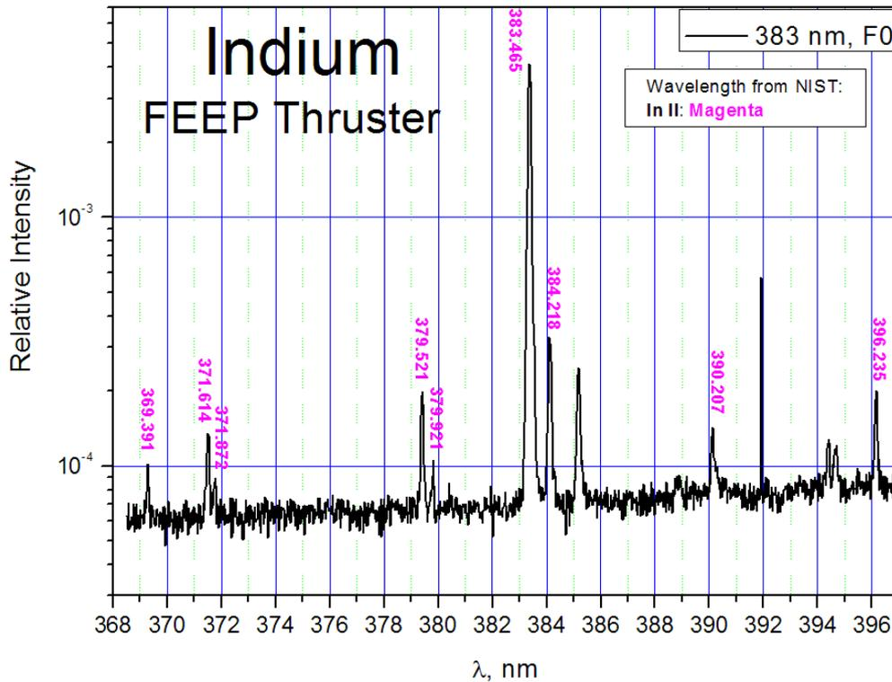
**Figure 8. Partial Indium spectrum of the FEEP Thruster.**
