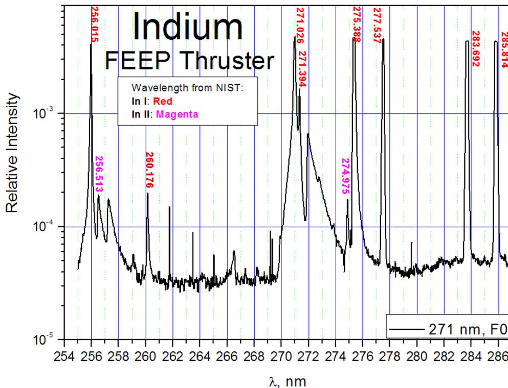
Figure 5. Partial Indium spectrum of the FEEP Thruster.
