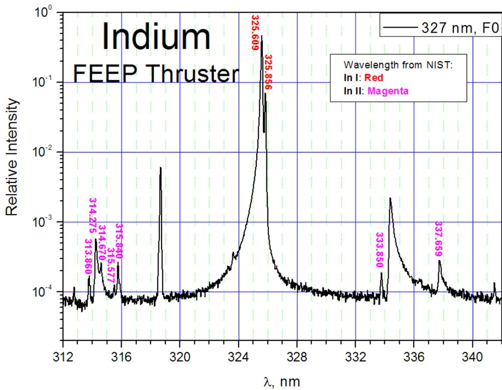
Figure 7. Partial Indium spectrum of the FEEP Thruster.
