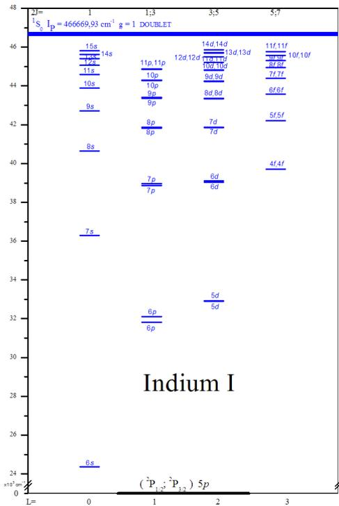
Figure 3. Grotrian Diagram of In I.
