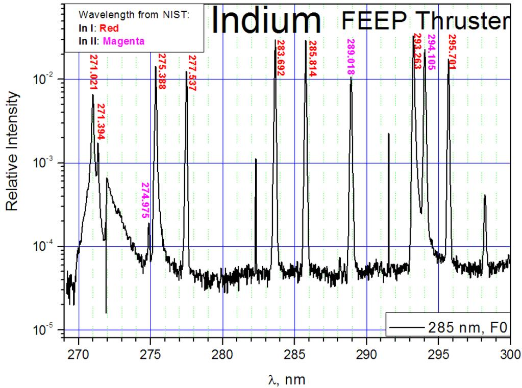
Figure 6. Partial Indium spectrum of the FEEP Thruster.
