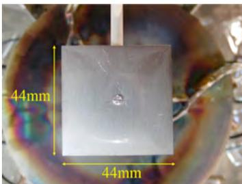
Figure 10. Ion collector.
