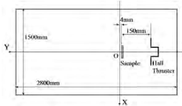
Figure 2. Setup configuration
