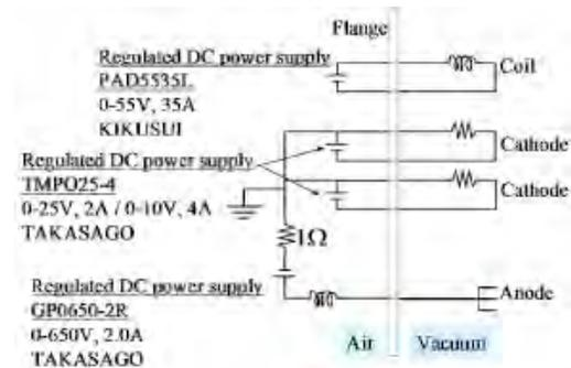
Figure 4. Electrical circuit of hall thruster.
