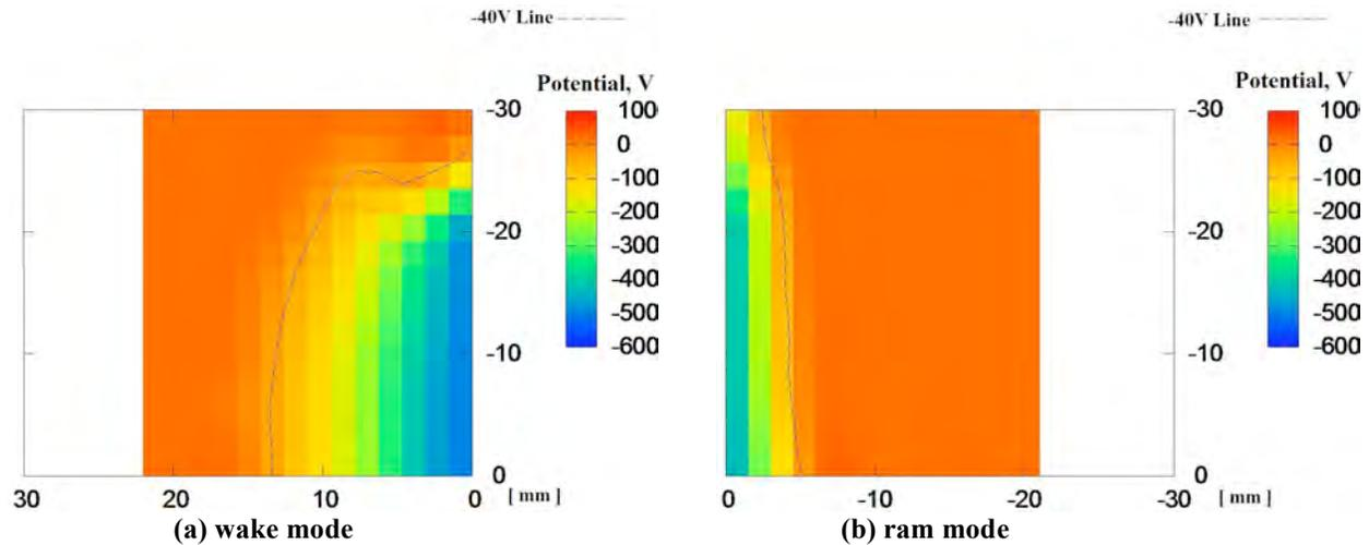
Figure 13. Potential distribution measured by emissive probe. Horizontal axis indicates the distance from collector plate.
