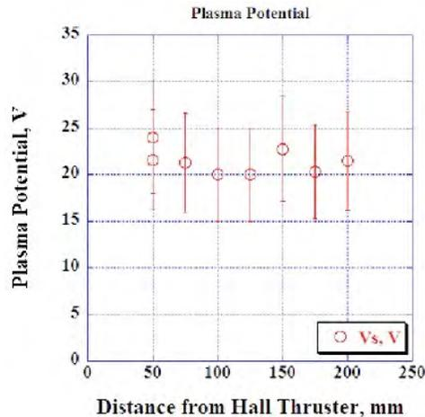
Figure 7. Plasma potential with respect to the chamber wall.
