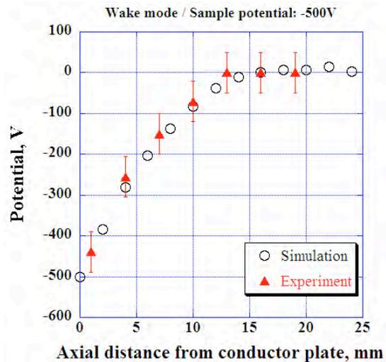
Figure 17. Comparison of plasma potential along the collector normal direction.
