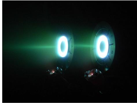
**Figure 6. HT-100 demonstration model (DM3) and engineering model (EM1) in cluster configuration for preliminary test**
