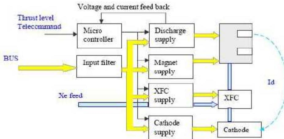
Figure 8. Small HET / PPU layout
