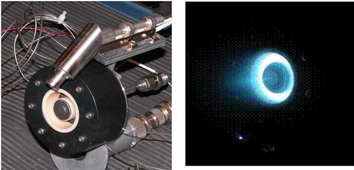
**Figure 4. HT-100 thruster development model (DM2), ©Alta**
