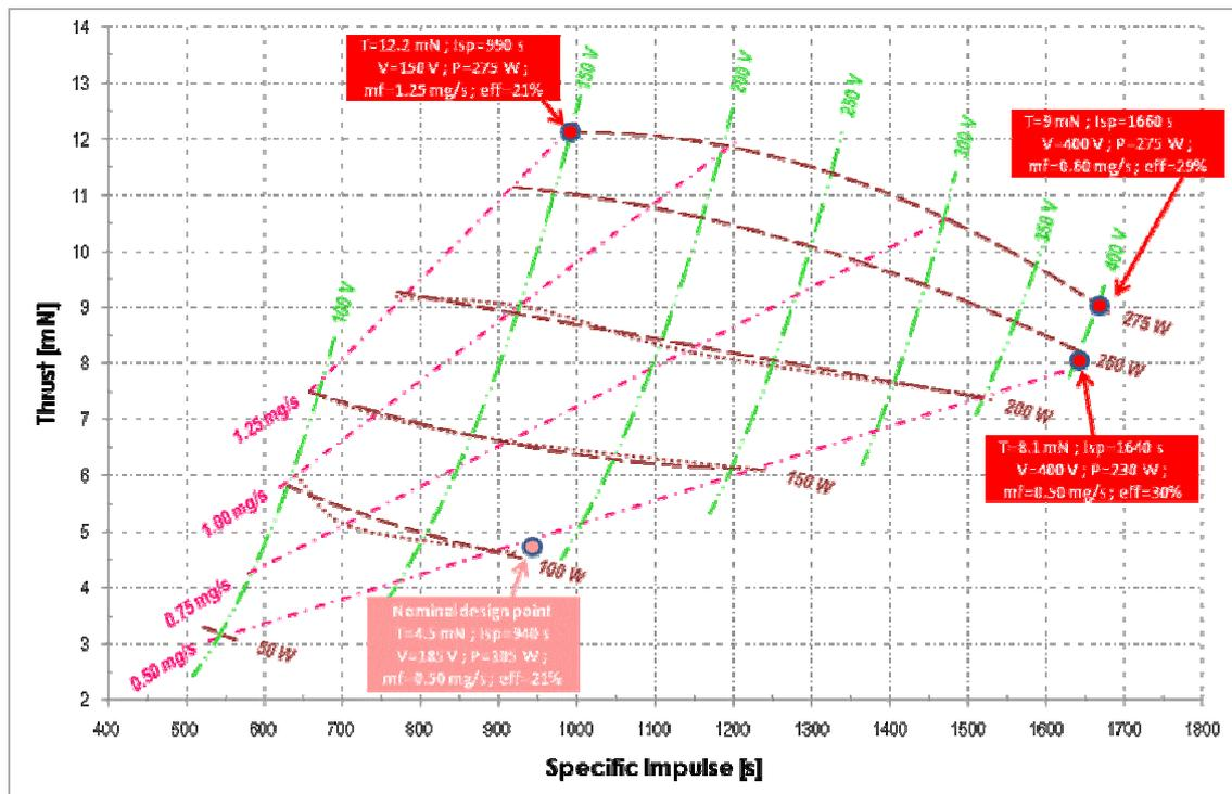
**Figure 5. HT-100 experimental performance map from 2007 test campaign**
