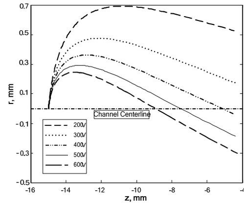
**Figure 7. *Xe* ion trajectories for the 200V to 600V discharge voltage.**
