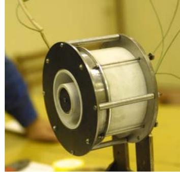
Figure 2. The picture of 1kW P70 Hall thruster.
