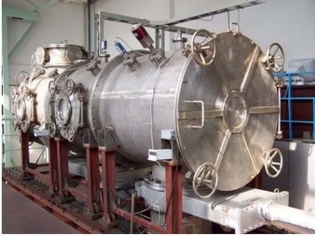
Figure 3. The vacuum chamber in HPPL.
