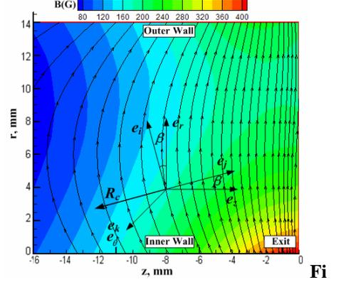
Figure 1. The distribution of two-dimensional static magnetic field.
