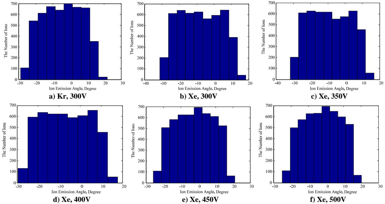
**Figure 5. The statistic of ion emission angle at the thruster exit plane.**
