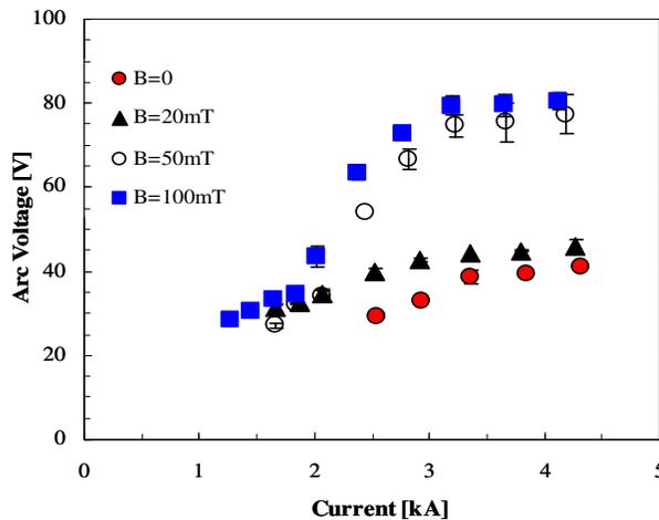
**Fig. 3: Configuration 0 electrical characteristics as a function of the applied magnetic field (100 mg/s of argon).**
