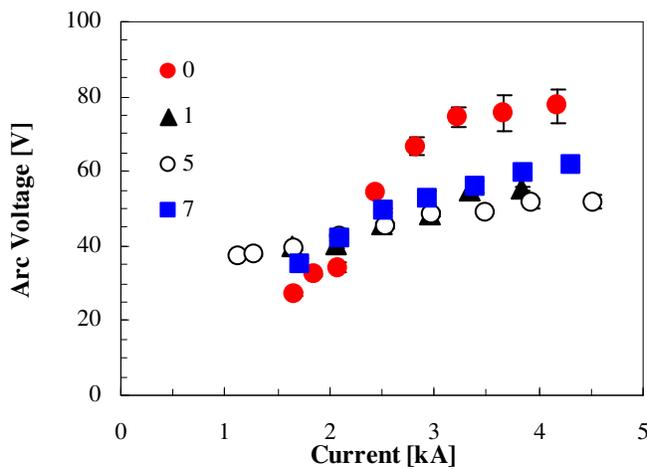
Fig. 9: Electrical characteristic comparison, 50 mT, 100 mg/s of argon. Conf. 0 vs Conf. 1, 5 and 7.
