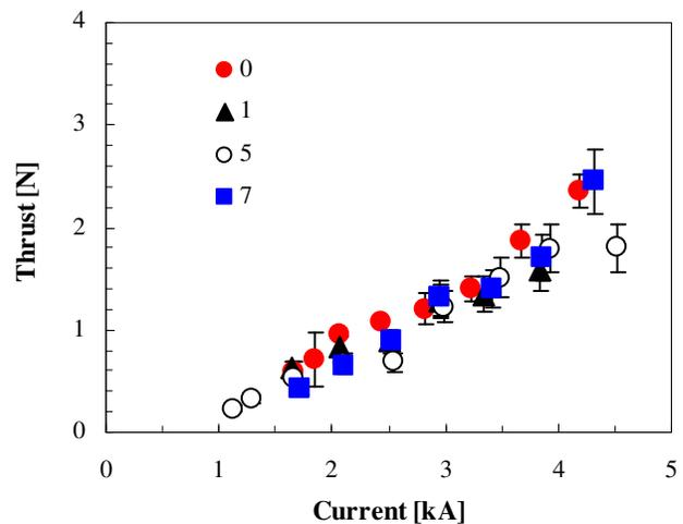
Fig. 10: Thrust comparison, 50 mT, 100 mg/s of argon. Conf. 0 vs Conf. 1, 5 and 7.
