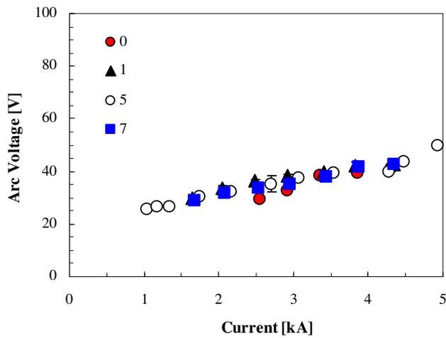
Fig. 5: Electrical characteristic comparison without applied magnetic field, 100 mg/s of argon. Conf. 0 vs Conf. 1, 5 and 7.
