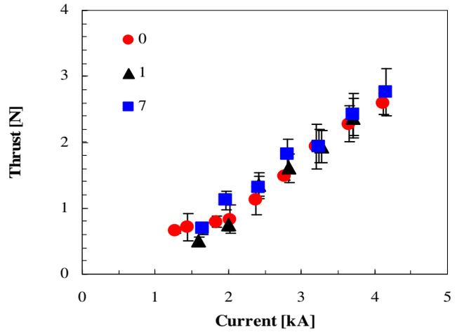
Fig. 12: Thrust comparison, 100 mT, 100 mg/s of argon. Conf. 0 vs Conf. 1 and 7.
