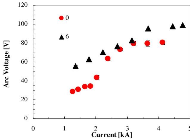
Fig. 13: Electrical characteristic comparison, 100 mT, 100 mg/s of argon. Conf. 0 vs Conf. 6.
