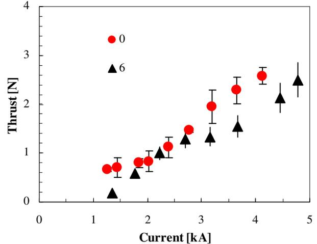
Fig. 14: Thrust comparison, 100 mT, 100 mg/s of argon. Conf. 0 vs Conf. 6.
