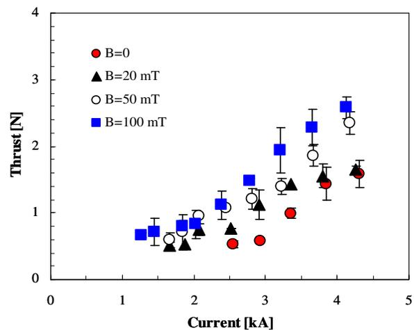
**Fig. 4: Configuration 0 thrust as a function of the applied magnetic field (100 mg/s of argon).**
