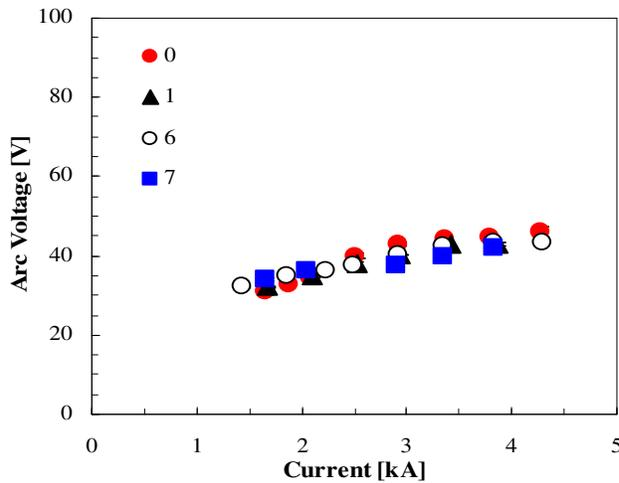
Fig. 7: Electrical characteristic comparison, 20 mT, 100 mg/s of argon. Conf. 0 vs Conf. 1, 6 and 7.
