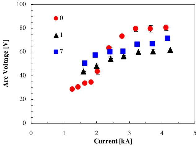
Fig. 11: Electrical characteristic comparison, 100 mT, 100 mg/s of argon. Conf. 0 vs Conf. 1 and 7.
