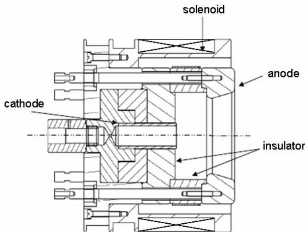
**Fig. 1: a cross section of the applied field MPD thruster investigated.**
