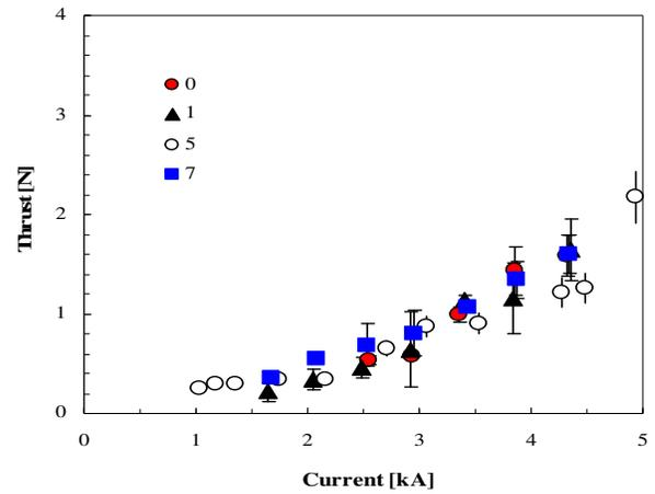
Fig. 6: Thrust comparison without applied magnetic field, 100 mg/s of argon. Conf. 0 vs Conf. 1, 5 and 7.
