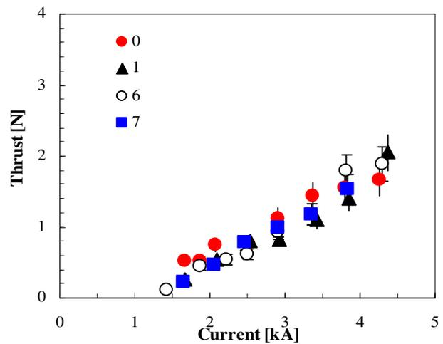
Fig. 8: Thrust comparison, 20 mT, 100 mg/s of argon. Conf. 0 vs Conf. 1, 6 and 7.
