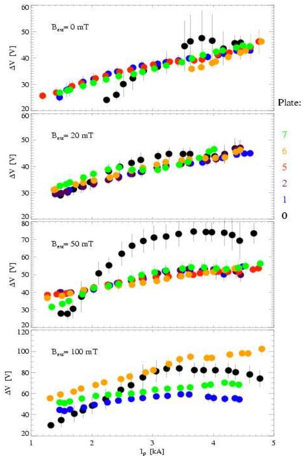
Fig. 9: Electrical characteristics of plasma discharges with various geometries of the inserted plate.
