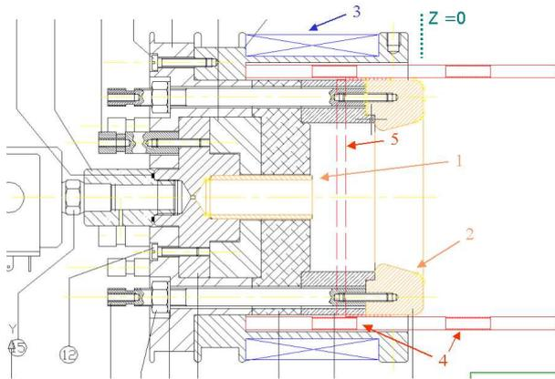
Fig. 1: Schematic of the MPD thruster and of the diagnostic system. 1) Cathode; 2) Anode; 3) External solenoid; 4) Magnetic pick-up probes; 5) Flux-probe
