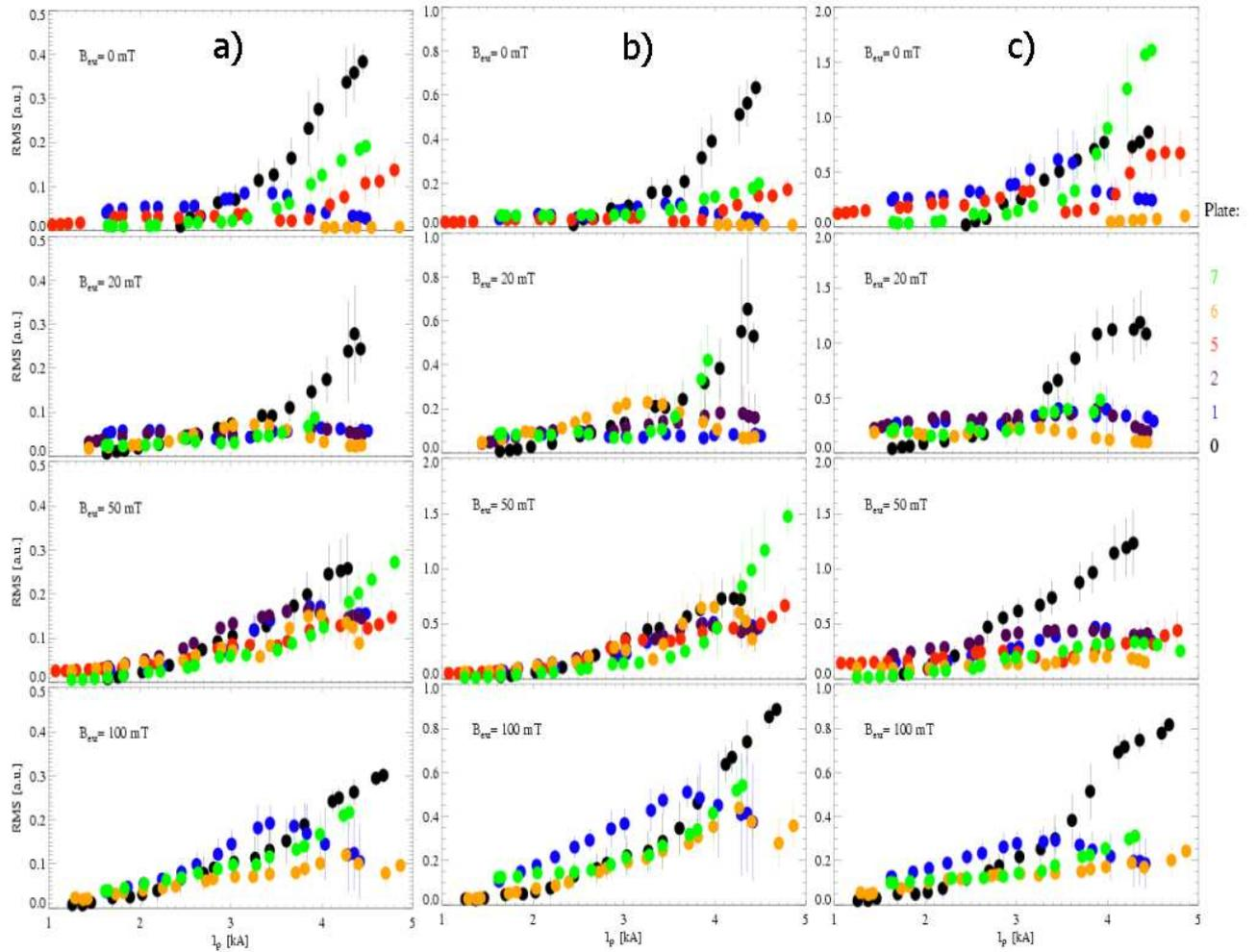
Fig. 6: RMS of magnetic signals: a) taken at  $z = -40$  mm, b) at  $z = 20$  mm, c) of the flux-probe, as a function of the plasma current, in different  $B_{ext}$  conditions and with the various plates for MHD control.
