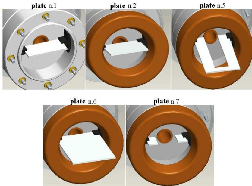
Fig.3: Schematic of the passive control systems (white plates) used.
