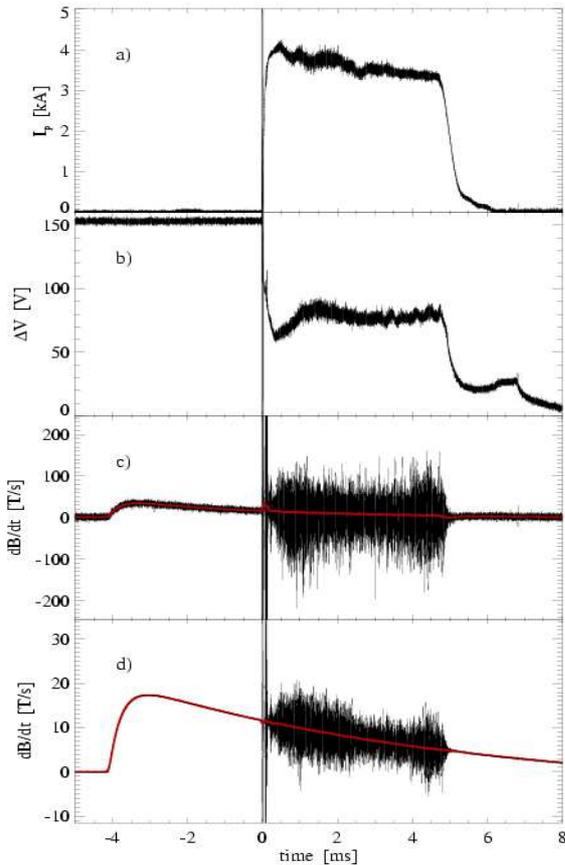
Fig. 4: Time history of a typical plasma discharge. a) Plasma current  $I_p$ ; b) Applied voltage  $\Delta V$ ; c) Pick-up coil signal (at  $z = -40$  mm); d) Flux-probe signal. Red lines are the low frequency component of the time-derivative of the  $B_z$  magnetic field.  $B_{ext} = 100$  mT in this case.
