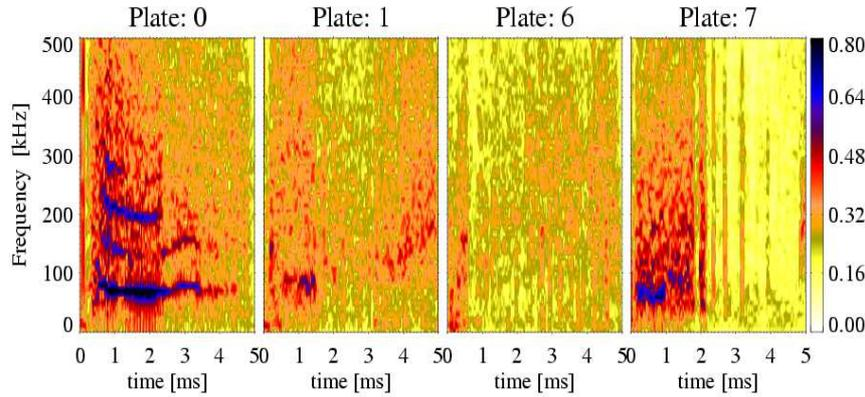
Fig. 7: Spectrograms of the flux-probe signal with various control systems. The color-scale is the same for all windows.  $I_p = 4$  kA,  $B_{ext} = 20$  mT in these cases.
