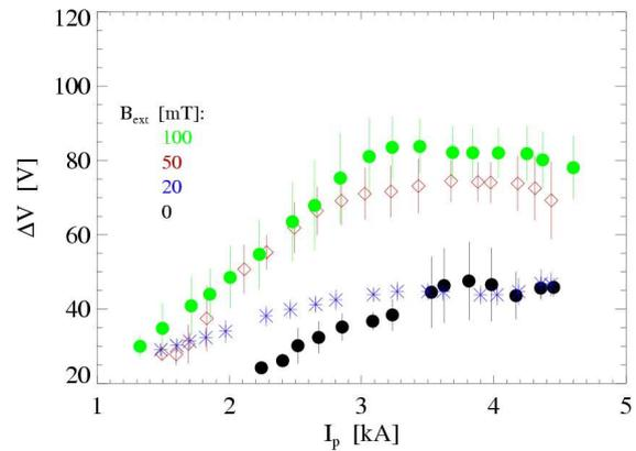
Fig. 2: Electrical characteristics of plasma discharges at different  $B_{ext}$  values.
