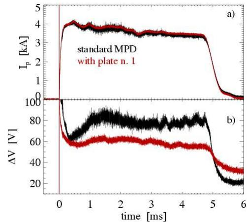
Fig. 9: a) Plasma current,  $I_p$ , and b) applied voltage,  $\Delta V$ , time evolution during discharges in standard MPD configuration (black curves) and with the insertion of one of the control systems used (red curves).  $B_{ext} = 100$  mT in these cases.
