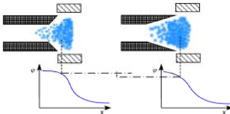
**Figure 8. Difference of ionization and ion acceleration between normal-type and divergent-type hollow anodes.**
