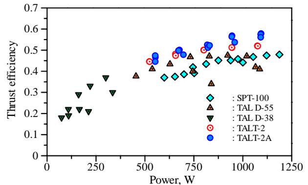
Figure 12. Thrust efficiency vs input power with our TALT series, and TAL D-series and SPT100.
