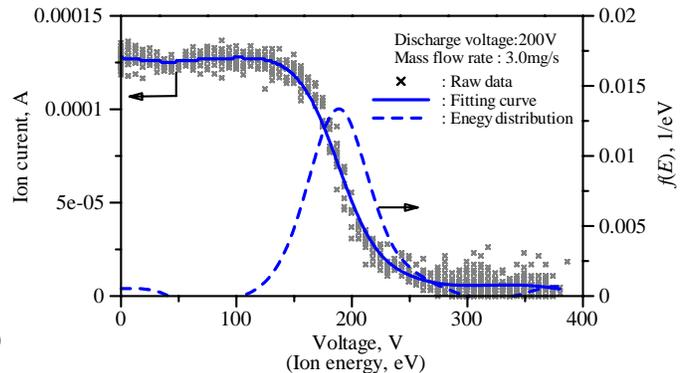
**Figure 5. Typical ion current profile and its energy distribution function by retarding potential analyzer.**
