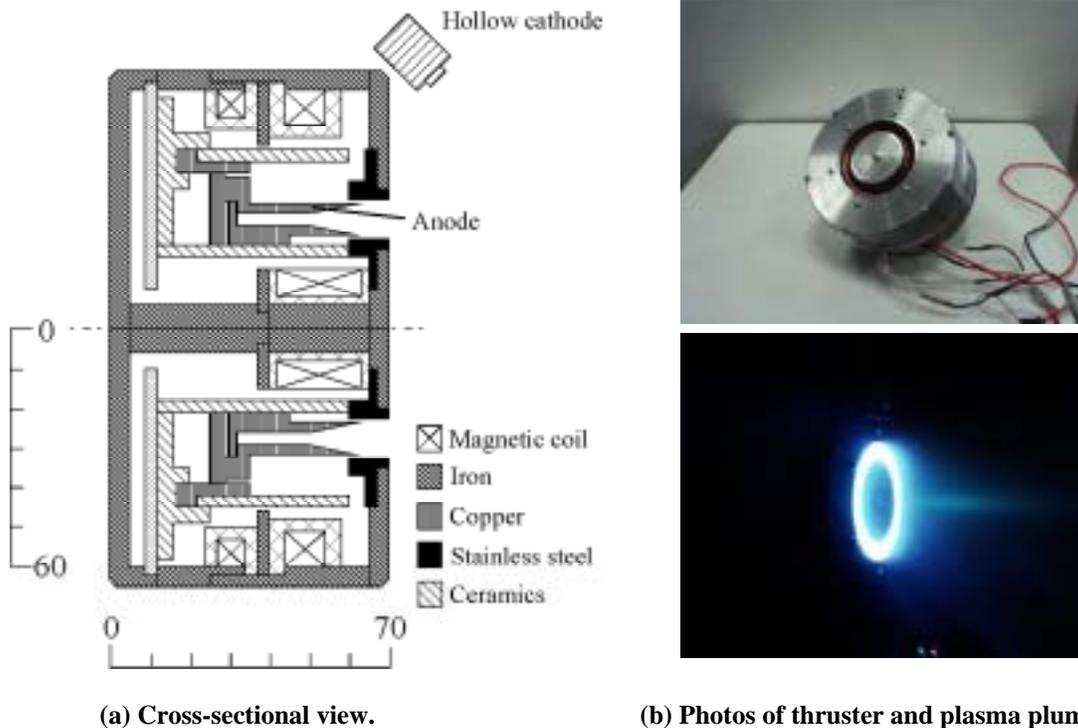
Figure 1. Cross-sectional view and photos of TALT-2 Hall thruster with divergent-type hollow anode.
