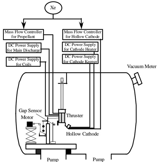
**Figure 3. Schematic view of experimental facility.**
