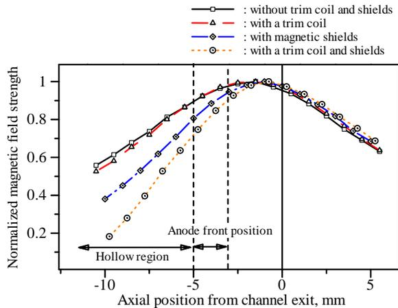
**Figure 2. Axial distributions of normalized Radial magnetic field strength.**
