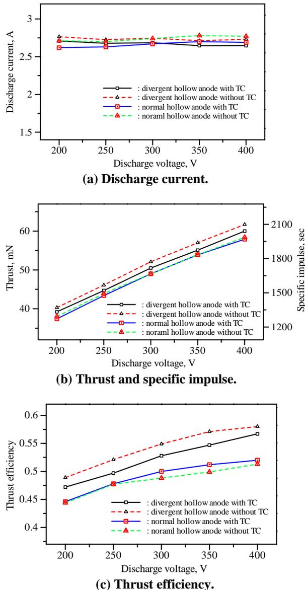
Figure 9. Performance comparisons between operations with normal-type and divergent-type hollow anodes.
