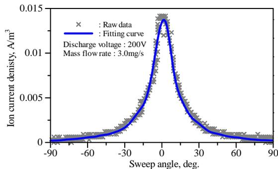
**Figure 4. Typical spatial distribution of ion current density by Faraday cup.**
