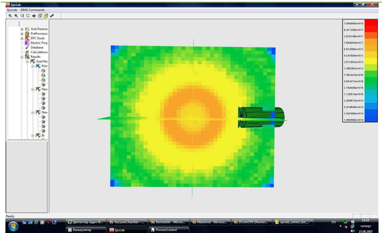
The primary ions distribution (parallel toward thruster exit face surface visualization)
