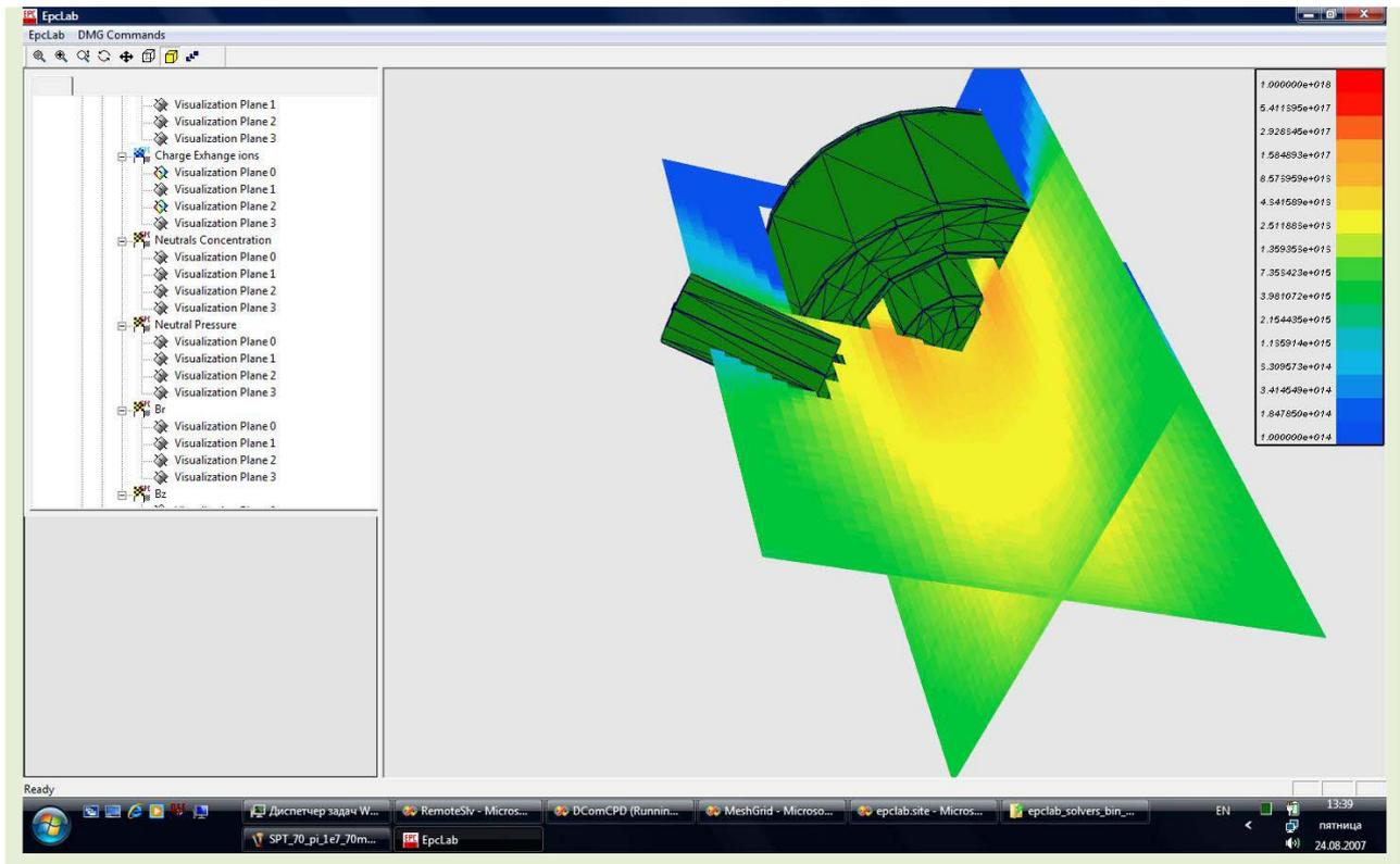
*The distribution of calculated CEX ion distribution with average velocity for 300K*
