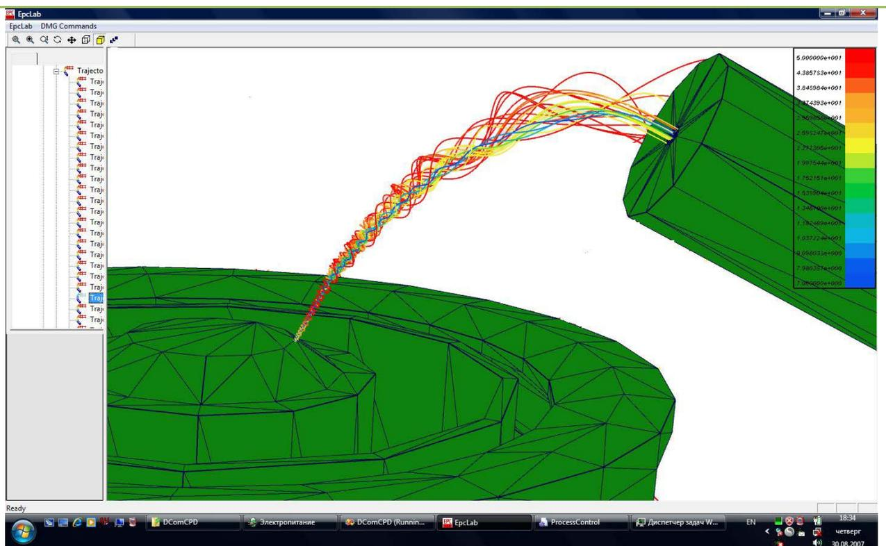
*Simulated beam of electrons with average start energy 12 eV (color correspond the energy in eV)*
