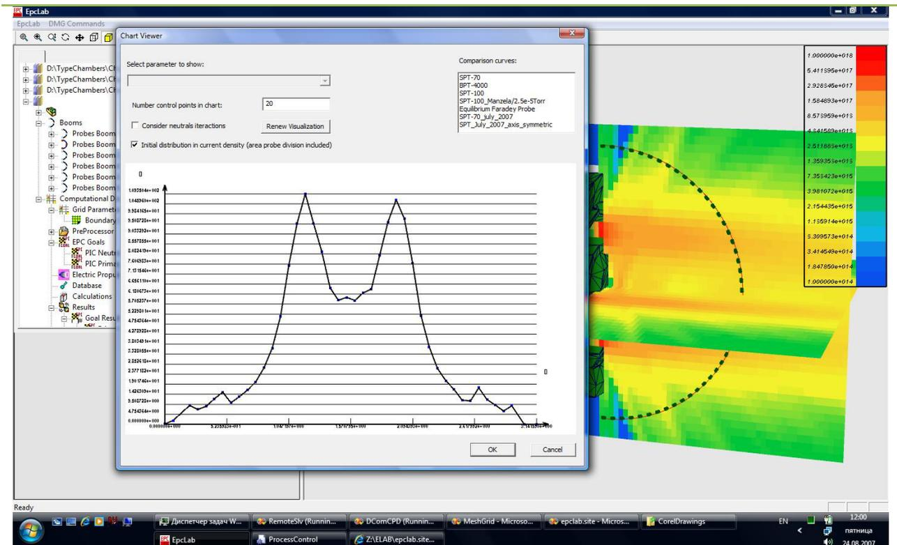
The calculated ion current on the boom with probes
