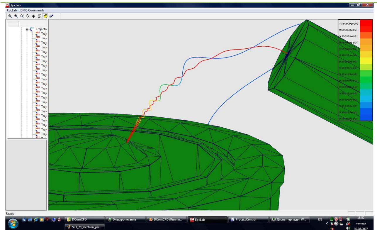
*Simulated interaction with neutral gas and primary ions. Relative distribution show decreasing of electron intensity in beam (color correspond the relative number of electrons in beam)*
