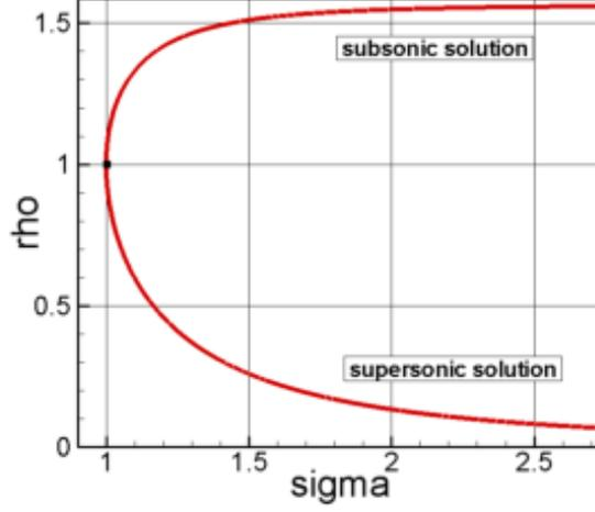
Figure 2. Subsonic and supersonic solutions for the density  $\rho$  as a function of the spherical radius  $\sigma$  for inlet sonic conditions. Both curves are plotted in dimensionless units.
