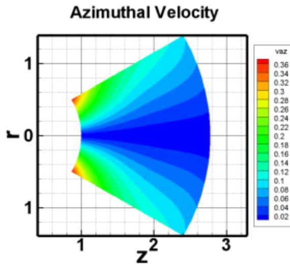
Figure 7. Contour plot of the azimuthal velocity function  $v_\phi$  for the example of thruster operation described in Sec. (VII).
