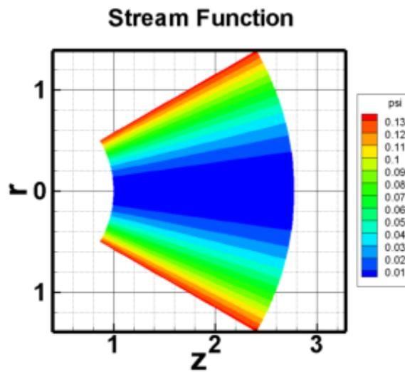
Figure 5. Contour plot of the stream function  $\psi$  for the example of thruster operation described in Sec. (VII).
