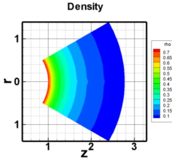
Figure 6. Contour plot of the density function  $\rho$  for the example of thruster operation described in Sec. (VII).
