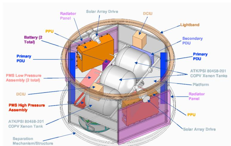
Figure 6. NEXT 1+1 SEP Module for Saturn Explorer.
