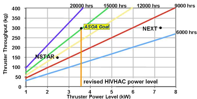
Figure 3. Throughput goal for the HiVHAC thruster.
