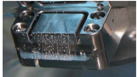
Figure 10. Slit emitter during one of the acceptance tests. The slit location is visible via the bubbles
