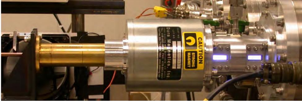
Figure 5. Cavity during operation with xenon. Plasma is visible through rectangular windows.
