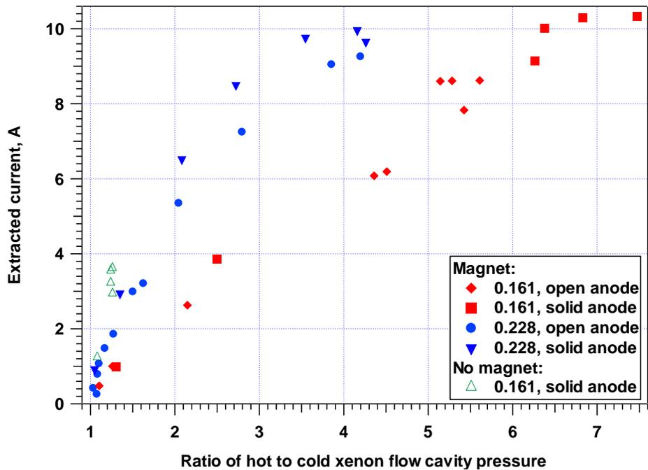
Figure 9. Extracted currents from Fig. 8, plotted against the ratio of cavity pressure during current extraction to cold flow (no plasma) cavity pressure.
