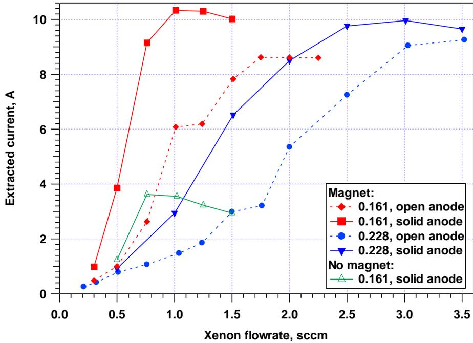
Figure 8. Anode current with 50 V bias, extraction aperture diameters of 0.161 and 0.228-in., with and without the magnet. Solid and open anodes refer to the presence or absence respectively of a 1.69-in. diameter plate attached to the downstream face of the anode.
