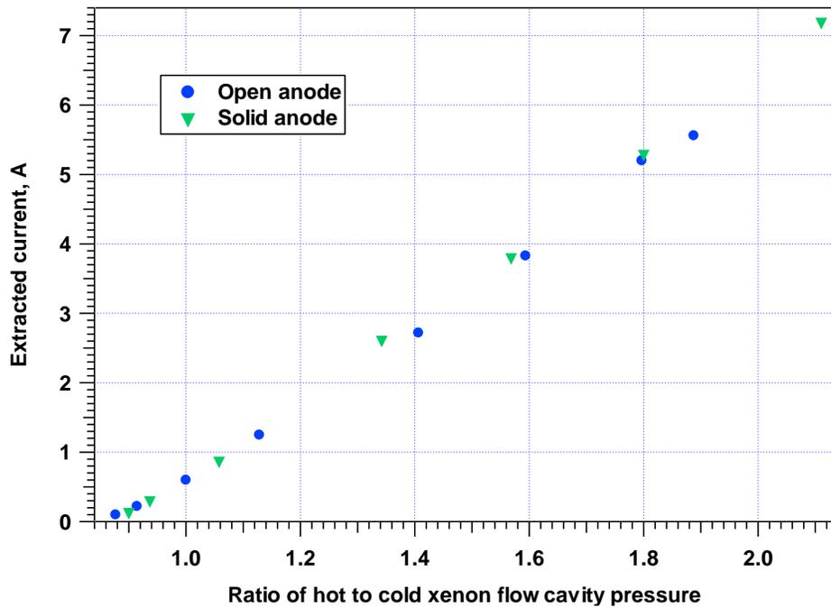
Figure 11. Extracted currents from Fig. 10, plotted against the ratio of cavity pressure during current extraction to cold flow (no plasma) cavity pressure.
