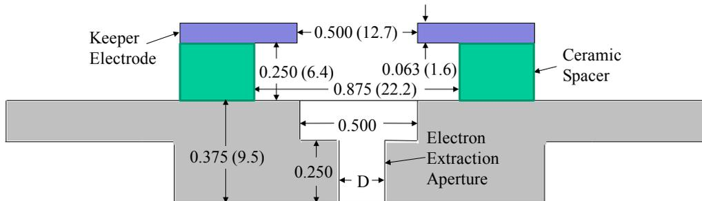
Figure 2. Enlarged section view of extraction aperture and keeper, dimensions in inches (mm).
