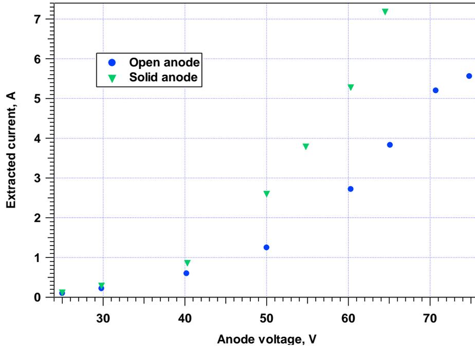
Figure 10. Extracted current at xenon flow rate of 1.0 sccm with 0.228-inch diameter extraction aperture.
