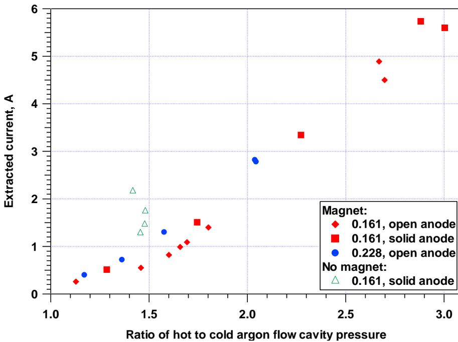
Figure 13. Extracted currents from Fig. 12, plotted against the ratio of cavity pressure during current extraction to cold flow (no plasma) cavity pressure.
