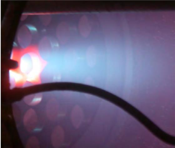
Figure 6. Extraction of approximately 9 A from xenon with 50 V bias on the “open” anode. Cavity aperture is out of view to the left, and is in line with the central anode aperture (glowing red).
