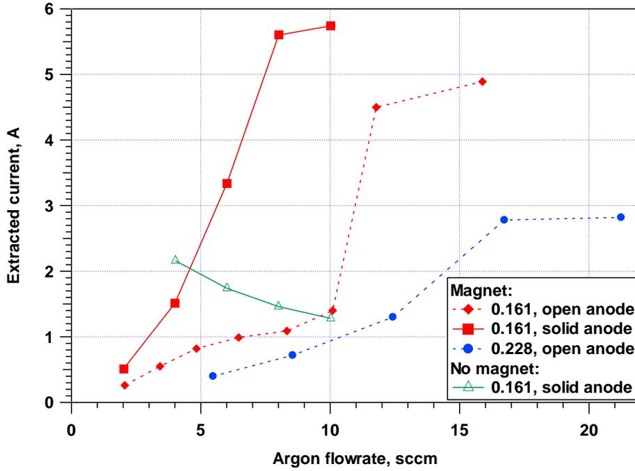
Figure 12. Anode current with 50 V bias, extraction aperture diameters of 0.161 and 0.228-in., with and without the magnet.
