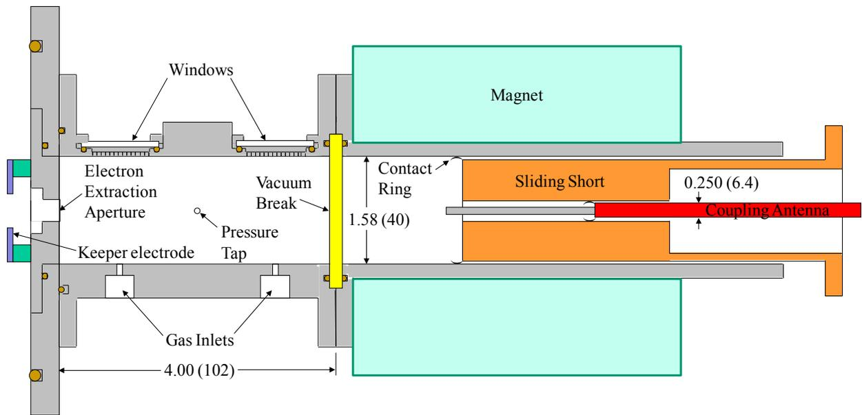
Figure 1. Section view of cavity, dimensions in inches (mm).
