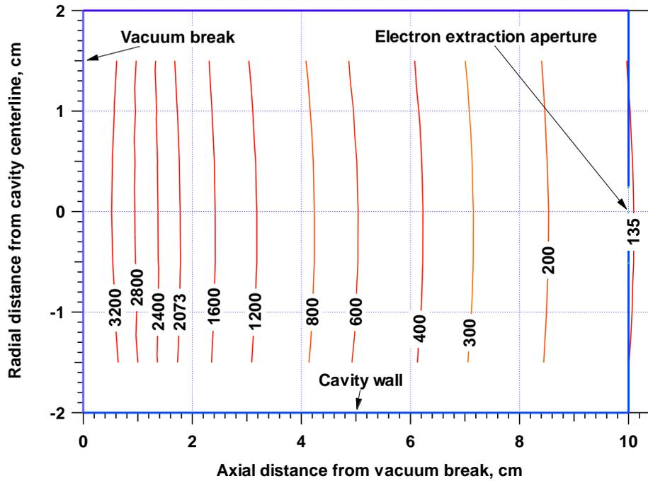
Figure 3. Contour plot of magnetic field magnitude (gauss) in plasma occupied region (outlined in blue). 2073 G contour shows resonant region at 5.8 GHz.
