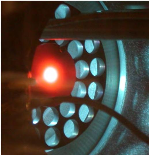
Figure 7. Extraction of approximately 10 A from xenon with 50 V bias on the “solid” anode.
