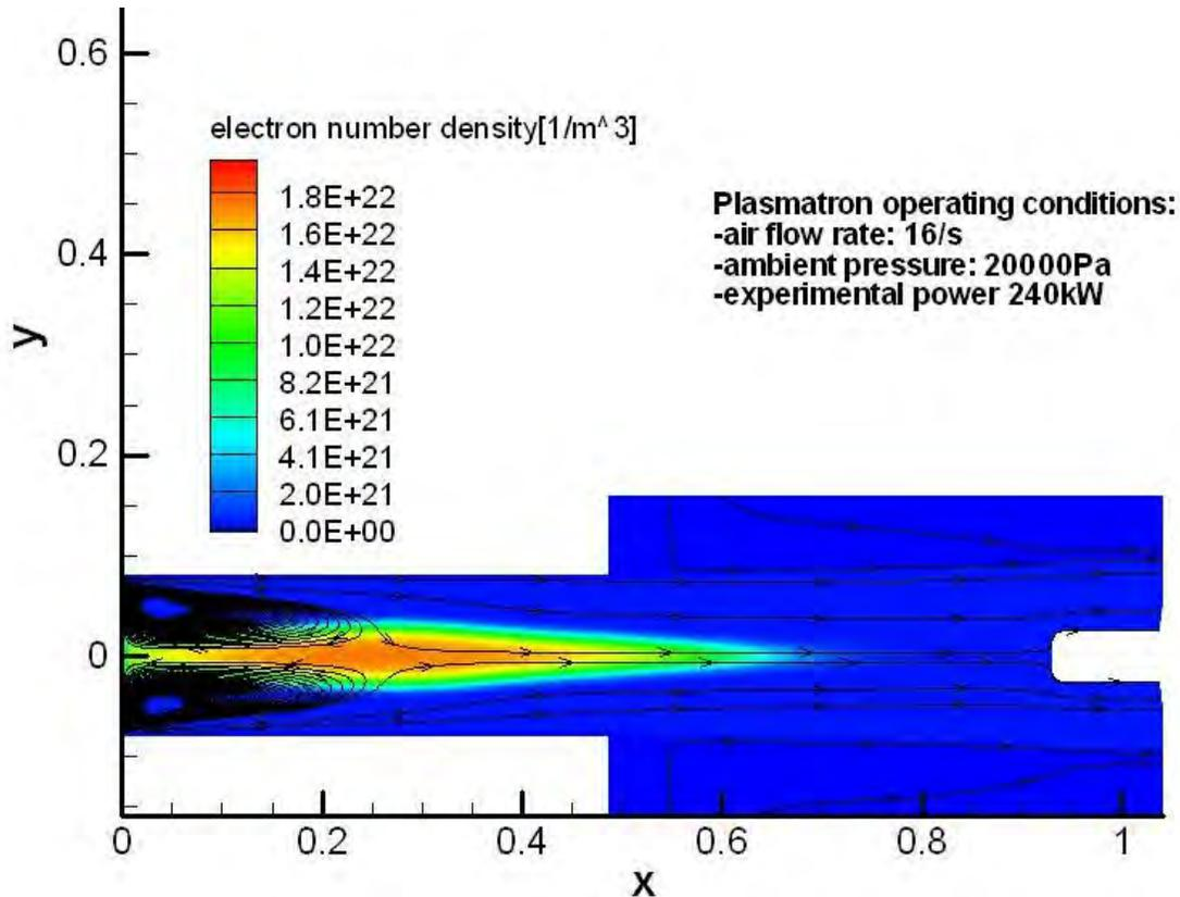
**Figure 1. CFD simulation of the electron plasma density in the VKI plasmatron. X and y values are in meters.**
