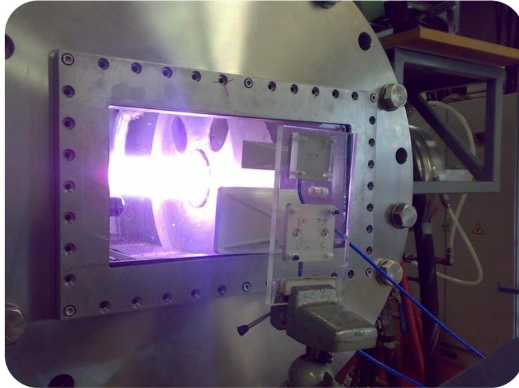
**Figure 6. Antenna setup showing Plasmatron in operation**
