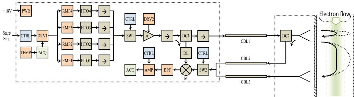
Figure key: PWR power supply, CTRL controller unit, TEMP temperature sensor, ACQ acquisition unit, DRV driver circuit, RMP ramp generator, HTO microwave source,  $\rightarrow$  microwave isolator, SW solid state switch, A power amplifier, DC directional coupler, DL delay line, CBL coaxial cable,  $\langle$  rectangular horn antennas, M downconversion mixer, BPF band pass filter, AMP signal amplifier.
