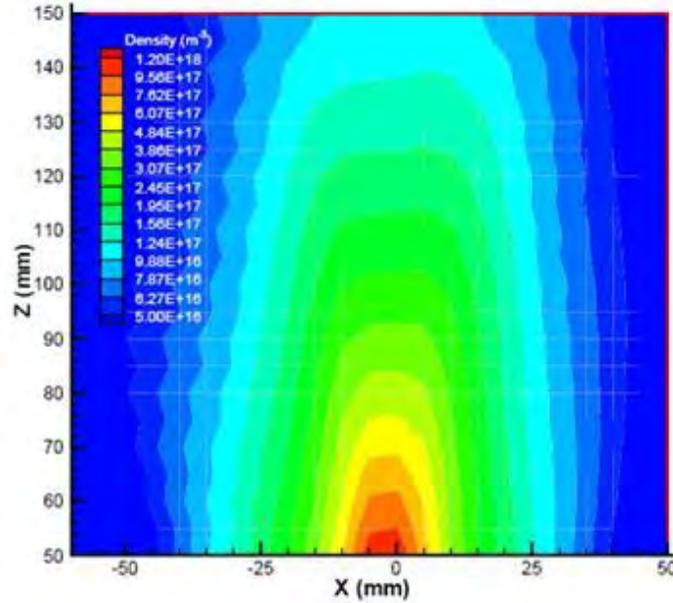
**Figure 2. Plasma density in the far-field plume of the BHT-200 thruster measured using a triple probe**
