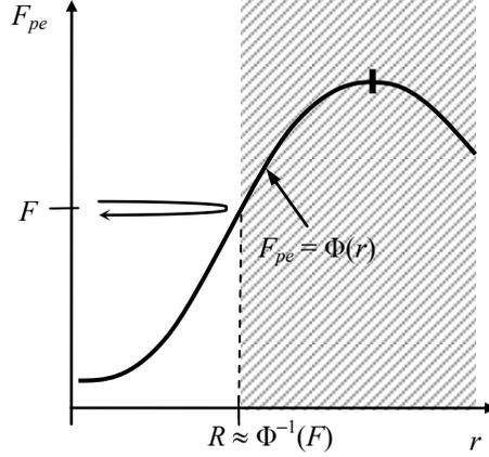
**Figure 3. Reflectometry principle**
