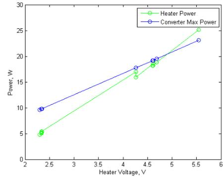
(d) This graph shows the heater's power consumption and the converter's power limit as a function of heater voltage. Near 5 V the heater attempts to draw more power than the converter can supply.
