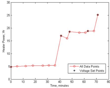
(c) Heater power as a function of time. Manual increases to the voltage using the trim are indicated with a star.
