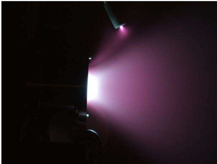
**Figure 10. DCFT during operation in the ASTROVAC.**
