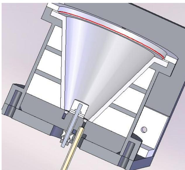
Figure 7. Solidworks model of new DCFT design.
