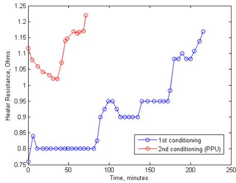
**Figure 12. Cathode resistance during conditioning.**
