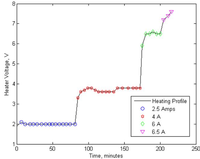
Figure 8. Heater voltage for given currents during conditioning.
