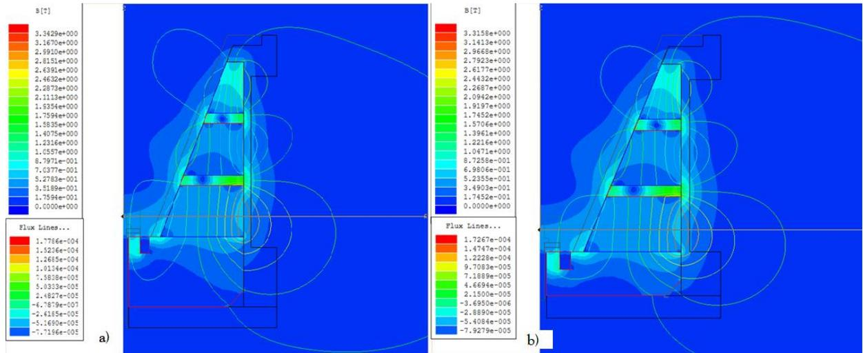
Figure 6. Magnetic topology on the r-z plane for the DCFT from (a) Previous Work and (b) the Current Study.<sup>18</sup> Found using Ansoft Maxwell SV software.
