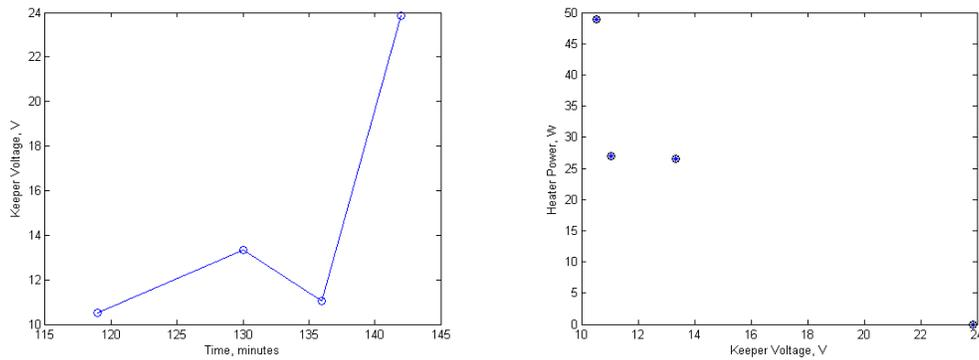
(a) Keeper voltage as a function of time. The keeper (b) Keeper voltage vs. heater power. As the heater shut off after reaching the maximum shown on the power was decreased, the keeper voltage steadily increased to the converter's limit.
