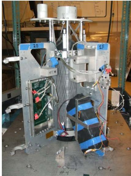
Figure 2. Mass mockup of the CASTOR satellite used for vibration testing.
