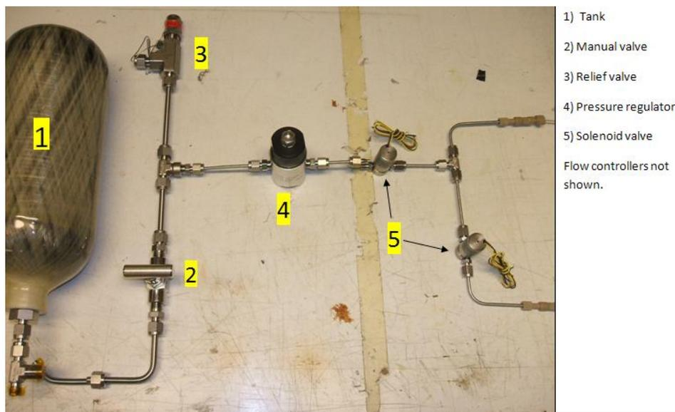
Figure 4. Propellant feed system for the DCFT.
