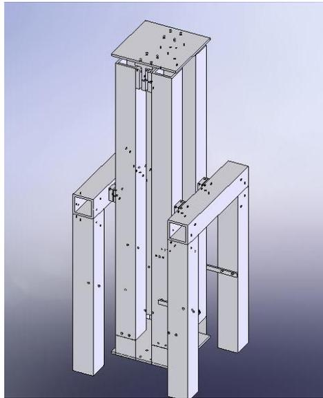
Figure 14. Solidworks model of thrust balance.
