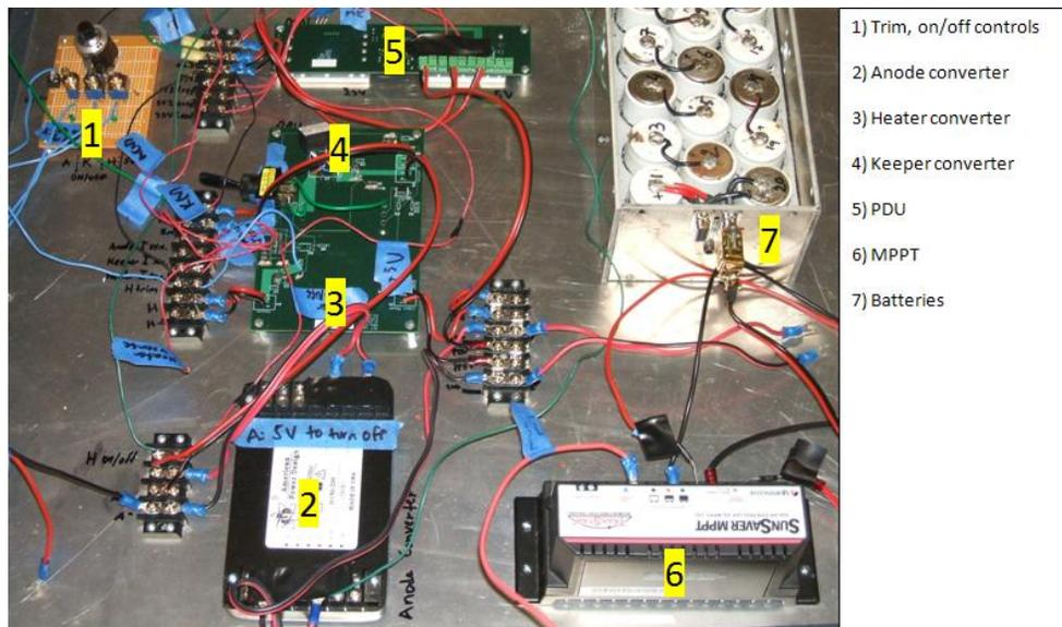
Figure 5. Current configuration of the PPU. Used with testing described in this paper.
