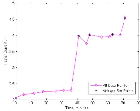
(b) Heater current as a function of time. Manual increases to the voltage using the trim are indicated with a star.
