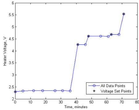
(a) Heater voltage as a function of time. Manual increases to the voltage using the trim are indicated with a star.
