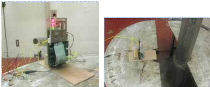
Figure 18. Gama rays exposure tests for OBC.
