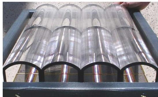
**Figure 3. SLA demonstrator in sunlight. Note light concentrated on PV stripes.**
