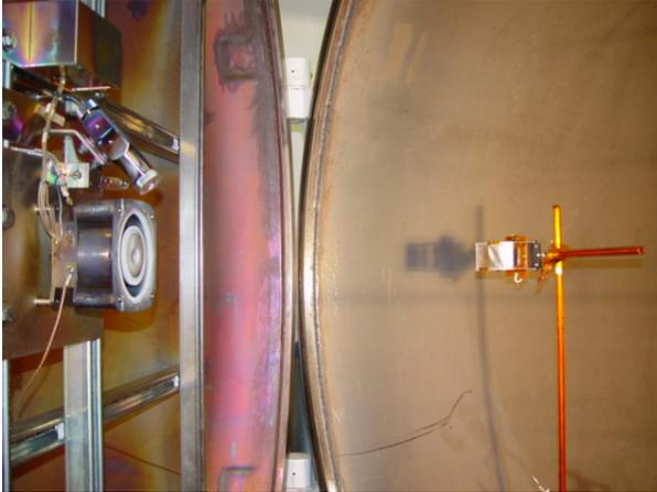
**Figure 10. SLA sample module in vacuum chamber with Hall thruster.**
