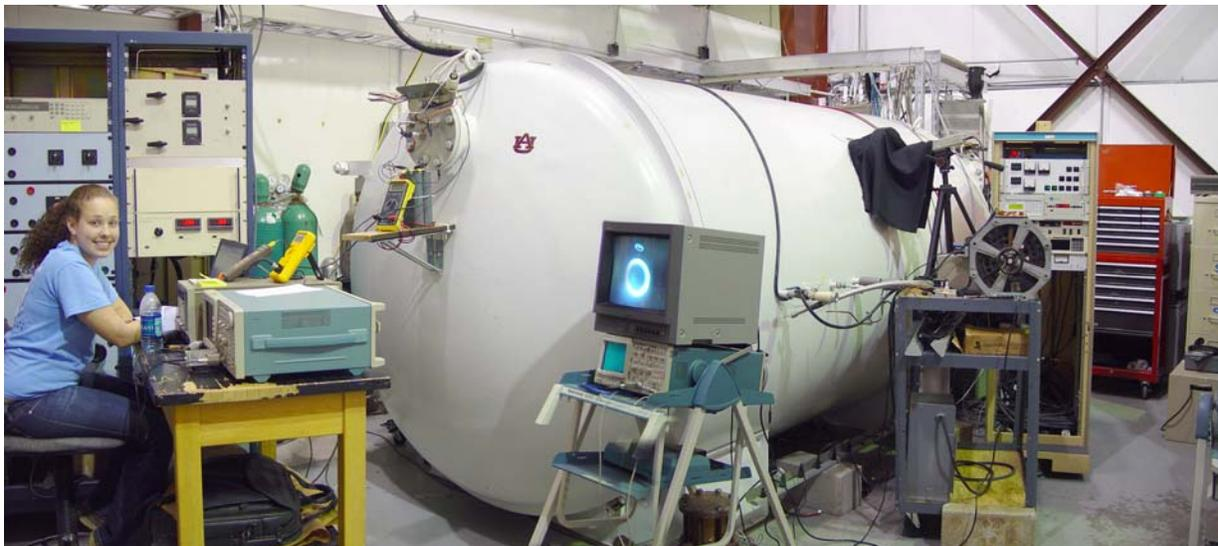
**Figure 7. Auburn University Space Research Institute's Electric Propulsion (EP) 9.2 m<sup>3</sup> test facility shown during testing of T-100 HET and SLA sample exposure.**
