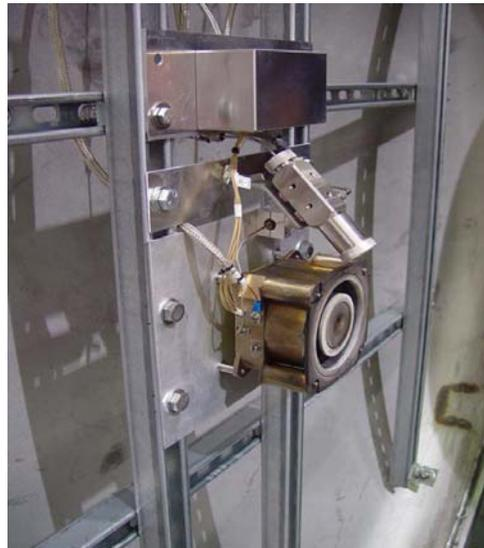
**Figure 6. T-100 Hall thruster and cathode..**
