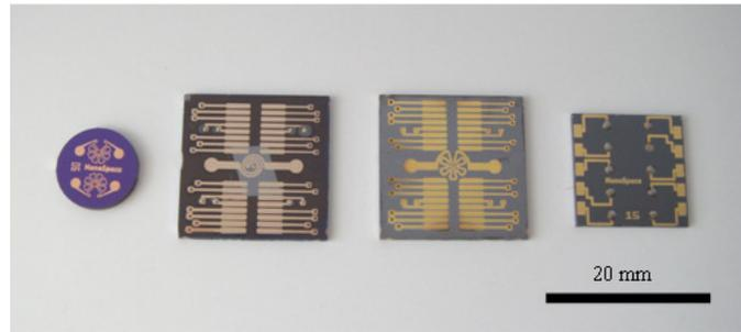
**Figure 16. MEMS-based fluid control components developed by NanoSpace. Total MEMS chip mass is about 10 grams.**
