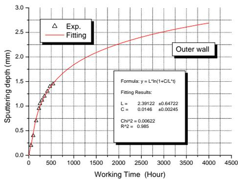
Fig.4 Extrapolation of external wall sputter erosion along with working time
