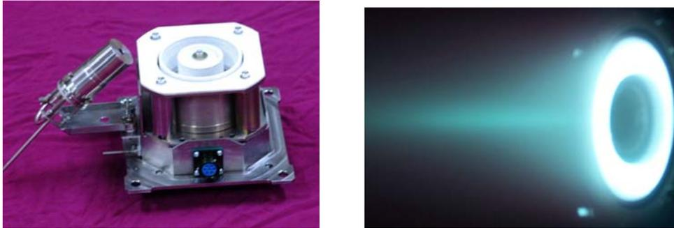
Fig.1 EM Hall thruster and its in operation
