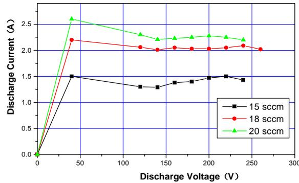
Fig.2 Volt-ampere characteristics of the thruster
