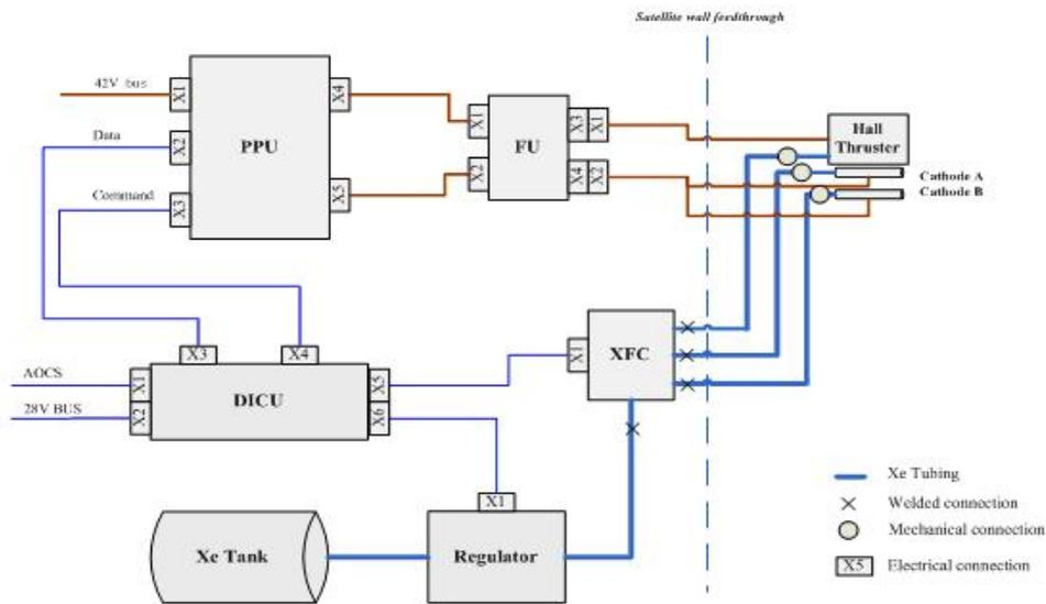
Fig.5 Scheme of Hall electric propulsion system
