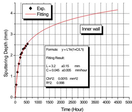
Fig.5 Extrapolation of internal wall sputter erosion along with working time
