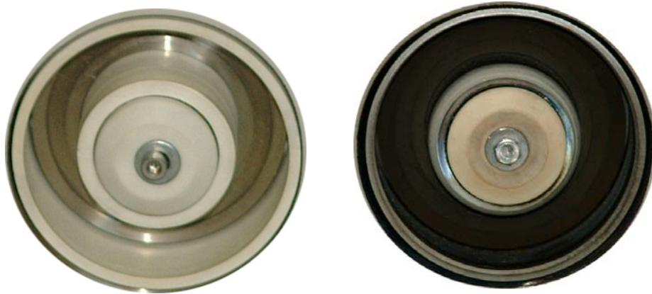
Fig.3 Appearance of discharge Chamber of thruster before & after 550h operation
