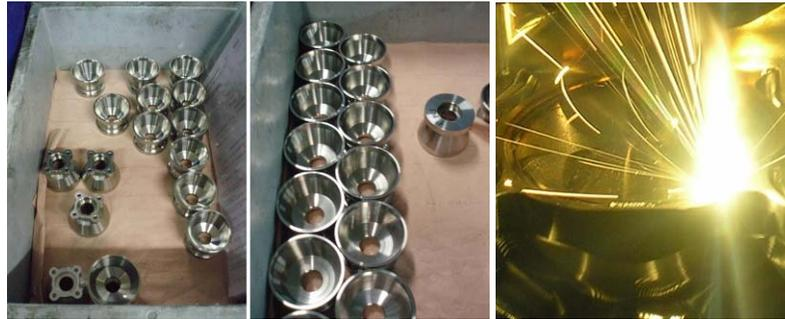
Figure 8. FEET Tank bodies manufacturing and welding
