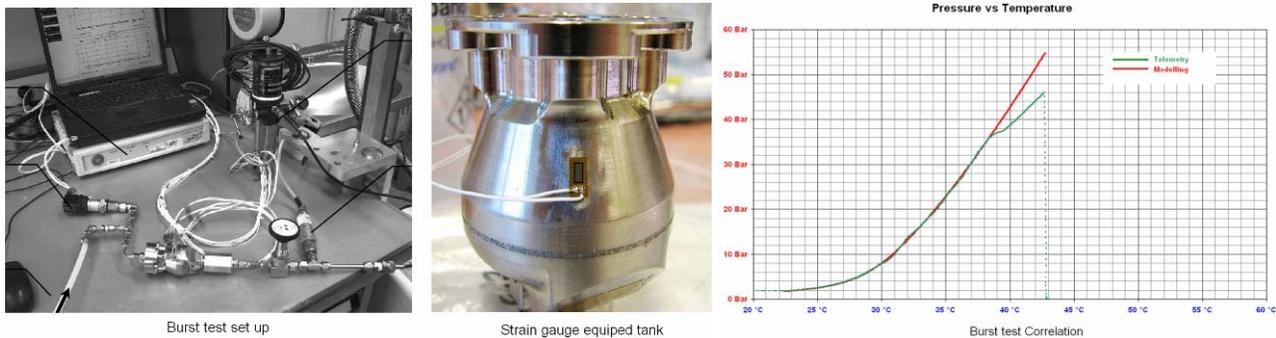
Figure 9. Mechanical and TSD functional Qualification. Proof and burst tests / Burst disc opening test
