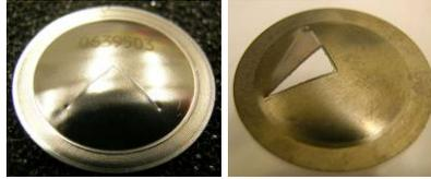
**Figure 5. Burst discs . closed and open**
