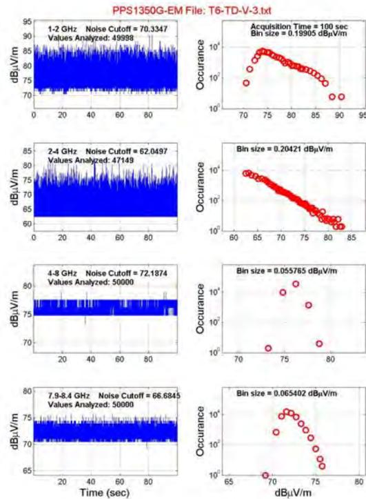
Figure 9. Log plots of 10 seconds of LSCX time domain data for the PPS1350-G EM operating in mode OP6. The left-side plots are the log amplitude electric field pulses; the corresponding right-side graph plots the distribution of these pulses
