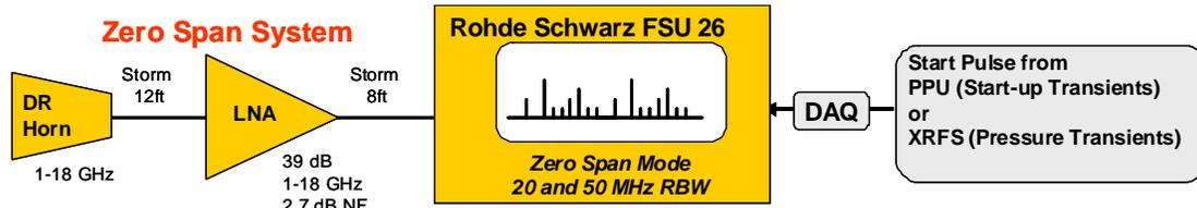
Figure 8. The Zspan time domain instrument.
