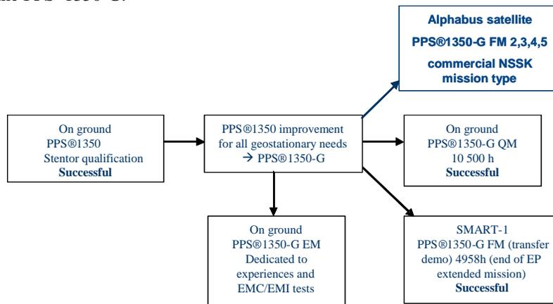
Figure 1. The PPS<sup>®</sup>1350-G qualification process.
