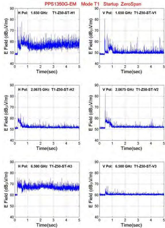
**Figure 12.** Log plots of zero span time-domain emission from the PPS1350-G EM thruster for three frequencies and two antenna polarizations. The emission in each panel in this figure was taken with a different thruster start.
