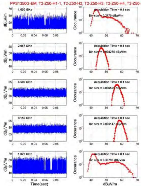
Figure 10. Log plots of 100 ms of zero span time domain data for five of the ten frequencies taken in horizontal polarization for the PPS1350-G EM operating in mode OP2. The left and right side panels are the same as those in Figure 9.
