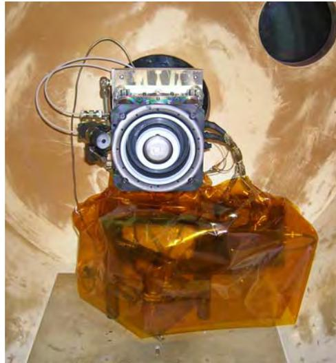
**Figure 3.** Photograph of PPS1350-G EM mounted in fiberglass tank. The cathode is mounted to the left, closest to the antenna placement.
