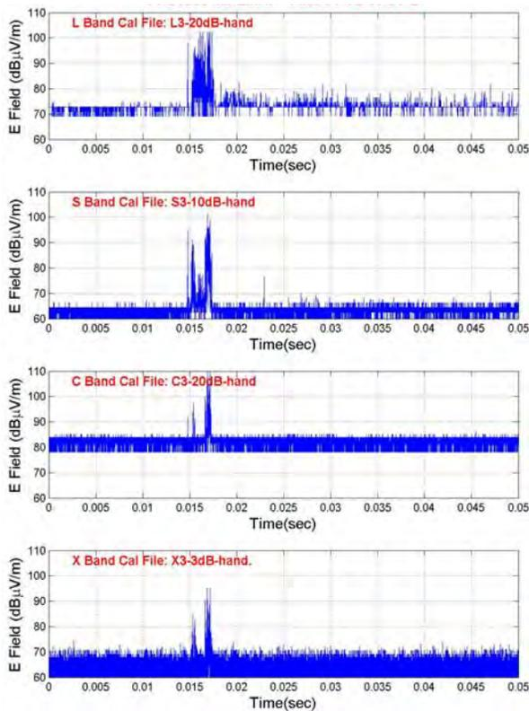
**Figure 11.** Log plots of horizontally polarized electric field emission from LSCX TD showing 50 ms of startup data from the PPS1350 MIr thruster. All in this panel data were taken with one thruster start.
