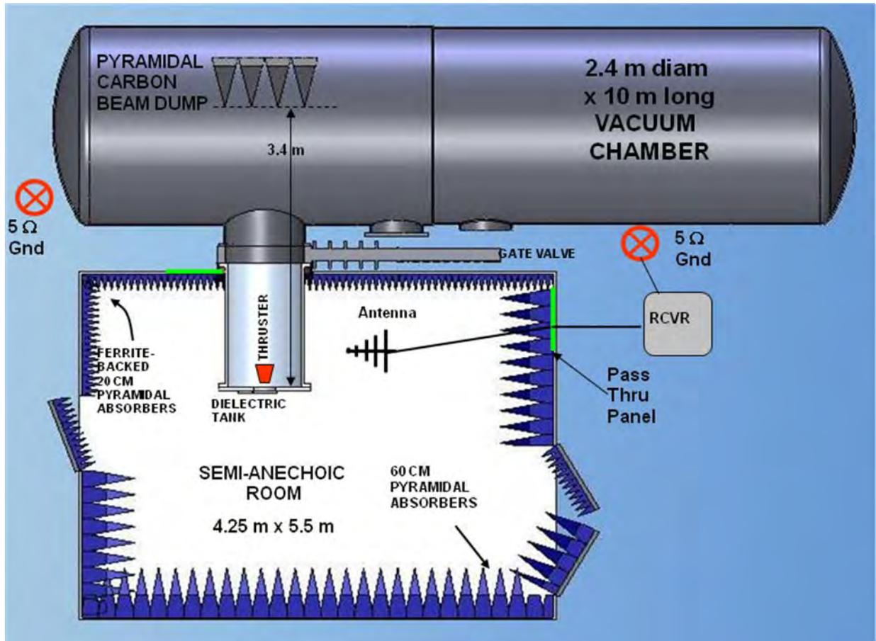
**Figure 2.** Scale Drawing of The Aerospace Corporation's EMC Facility.
