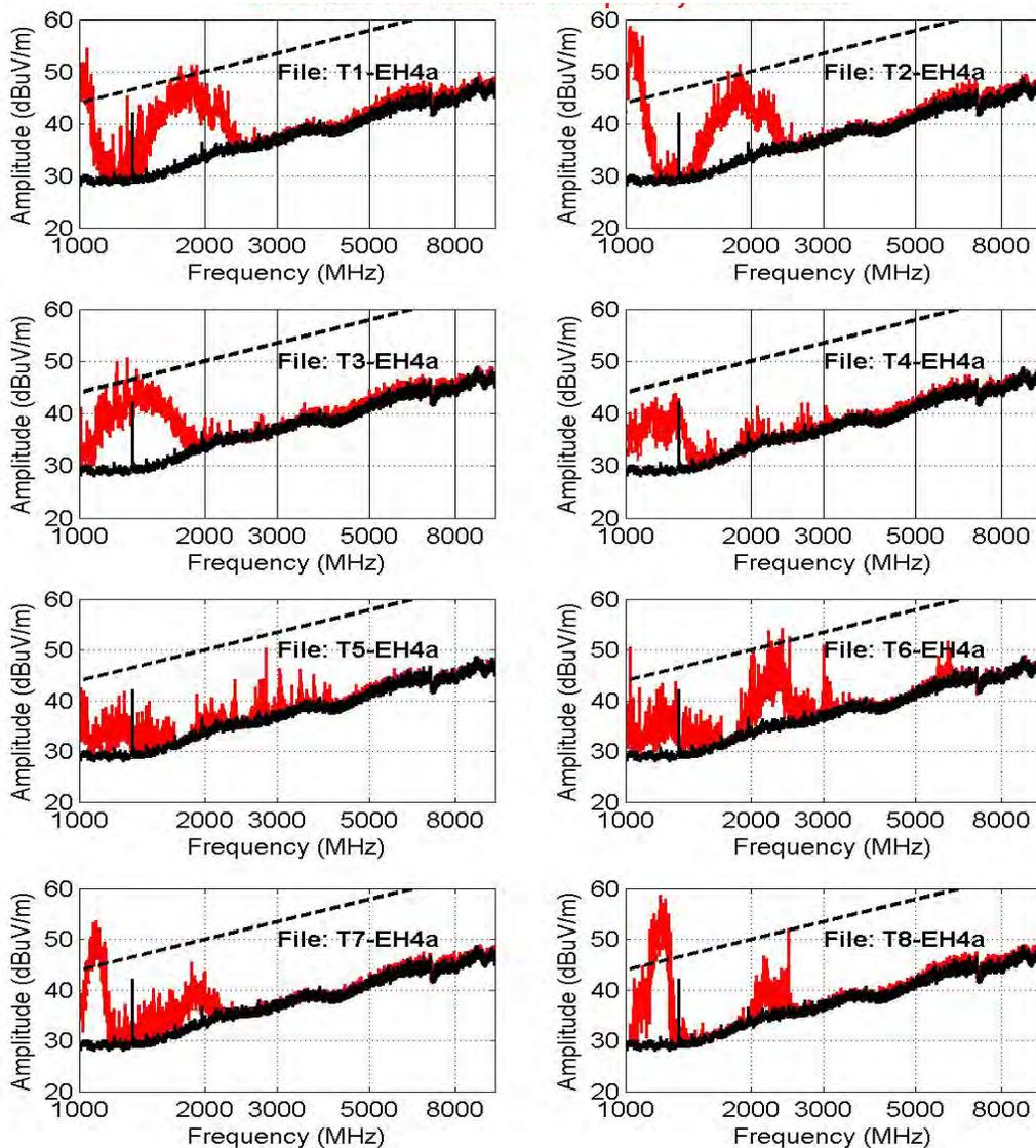
**Figure 5.** Variation in the spectra as a function of operation mode for OP1–OP8 for horizontal polarization and the PPS1350-MIr thruster. Blank curve is thruster off; red curve is thruster on, dashed line is MIL-STD-461 limit.
