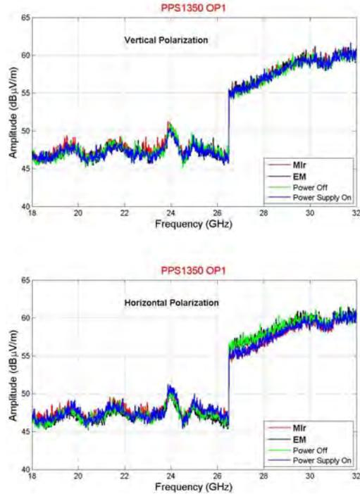
**Figure 6.** Spectra from 18 kHz–32 GHz (vertical polarization, upper panel, horizontal polarization, lower panel) for the PPS1350 Mir and the PPS1350-G EM thrusters
