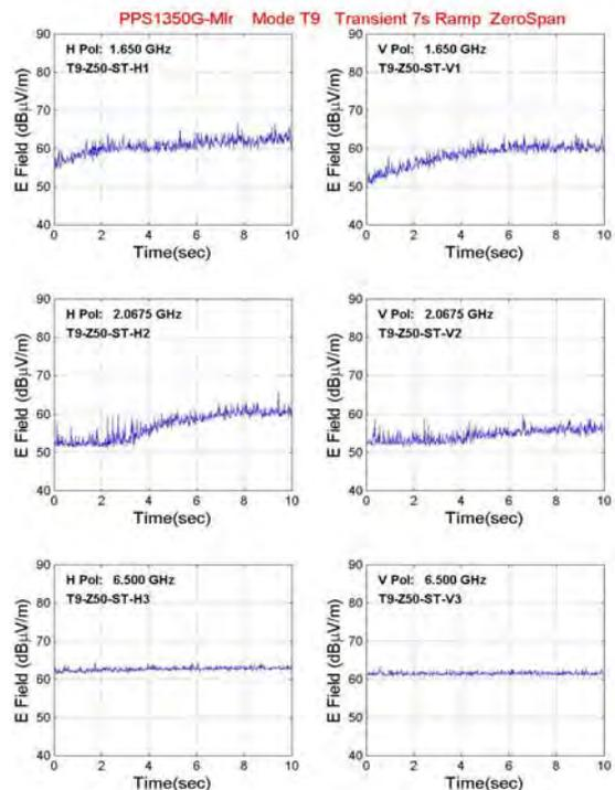
**Figure 14** Log plots of Zspan instrument data from the PPS1350 Mir thruster during an 100V increase in anode potential.
