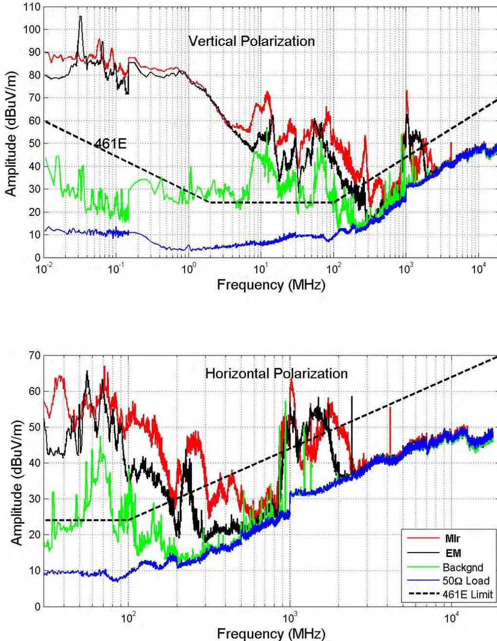
**Figure 4.** Spectra from 10 kHz–18 GHz (vertical polarization, upper panel) and 30 MHz – 18 GHz (horizontal polarization, lower panel) for the PPS1350 MIR and the PPS1350-G EM thrusters.
