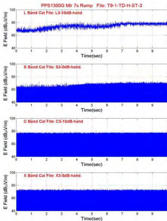
**Figure 13** Log plots of horizontally polarized emission from the PPS1350 Mir thruster during a 100V increase in anode potential.
