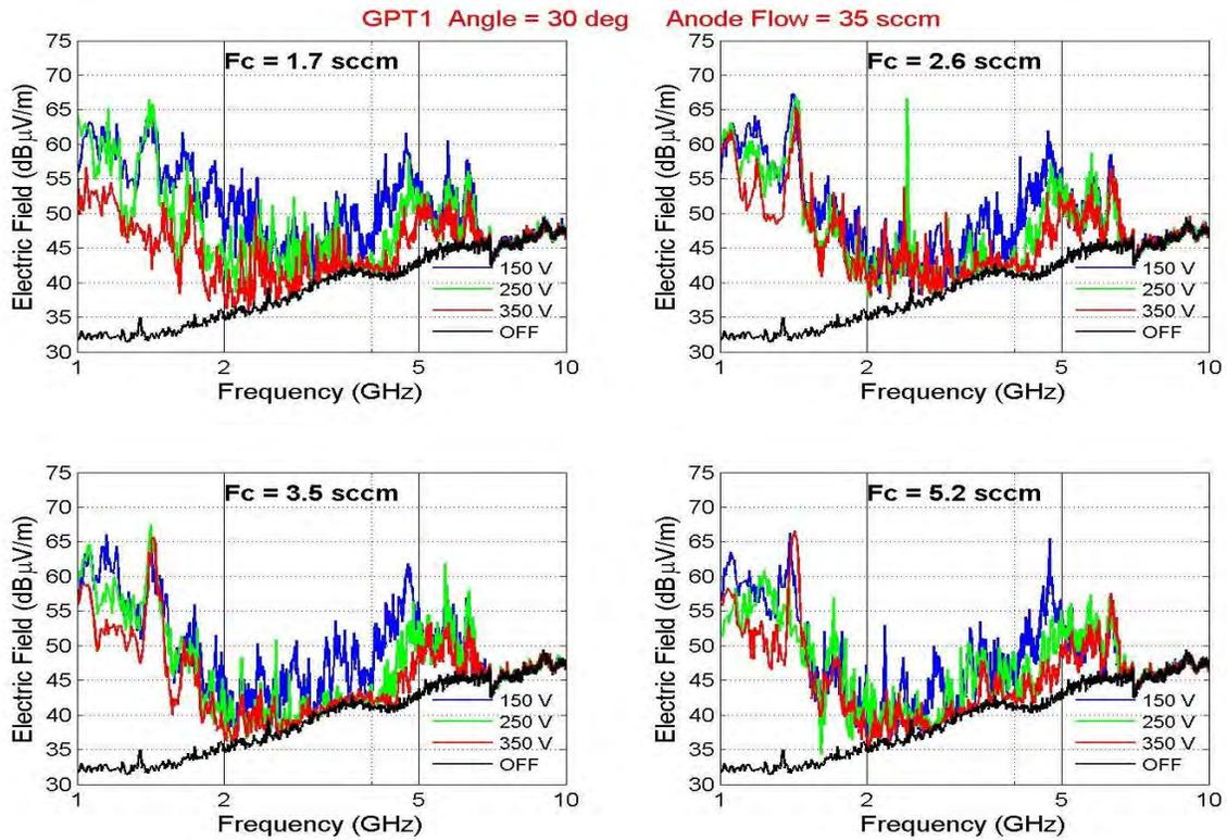
**Figure 3.** 1-10 GHz emission for an anode flow rate of 35 sccm, 4 cathode flow rates, and 3 discharge voltages. Magnetic field is the same for all spectra. The black line is the background emission (thrustor unpowered).
