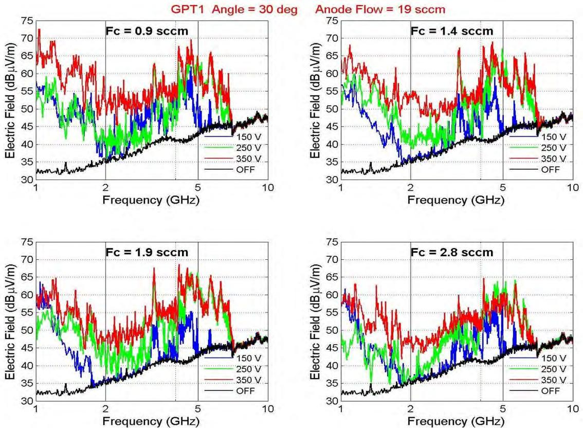
**Figure 4.** 1-10 GHz emission for an anode flow rate of 19 sccm, 4 cathode flow rates, and 3 discharge voltages. Magnetic field varied with discharge voltage. The black line is the background emission (thrustor unpowered).
