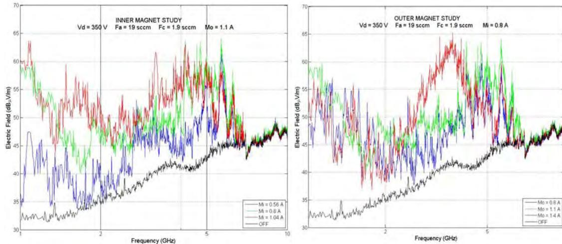
**Figure 6.** Spectra for differing values of the magnetic field. The left panel shows 3 spectra holding the outer magnet coil current at 1.1 A while increasing the inner coil current from 0.56 A to 1.04 A. The right panel shows 3 spectra where the outer coil current is varied from 0.8 A to 1.4 A while holding the inner coil current at 0.8A.
