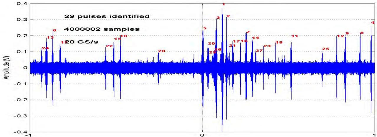
**Figure 7.** A 200- $\mu$ s trace showing the individual pulses emitted from a Hall thruster in L-band.
