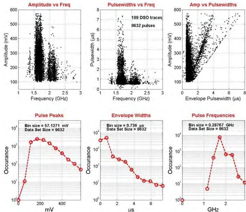
**Figure 8.** Analysis of 109 traces of the type shown in Figure 7. These plots display the characteristics of the individual pulses (upper three plots) and their statistical properties (lower three plots).
