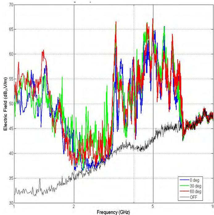
Figure 2. LSC spectra as a function of cathode angle for thruster mode 8.
