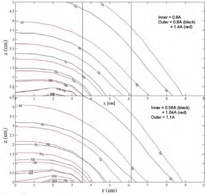
**Figure 5.** Magnetic field plots for 4 magnet coil currents. The vertical axis is distance from thruster face; horizontal axis is distance from thruster centerline. Two vertical lines mark the position of thruster channel. Cathode orifice is at  $r = 10$  cm,  $z = 0$  cm.
