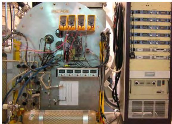
**Figure 5. Photograph of VF-8 Bell jar 2, xenon feed system, and the power console used in EM-1 testing.**
