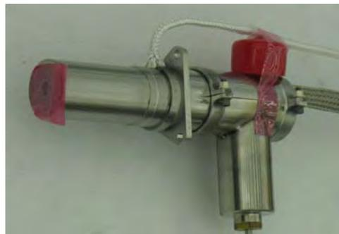
**Figure 4. Photograph of the HiVHAc EM hollow cathode assembly.**
