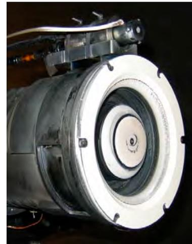
**Figure 2. Photograph of the NASA-103M.XL thruster after 4,731 hours of testing at 700 V.**
