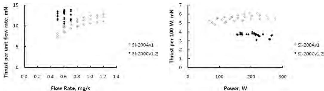
**Figure 6. Performance comparison between the SI-200Av1 and the SI-200Cv series in the voltage range of 200-250 V. Full markers denote the SI-200Cv-series and empty markers denote the SI-200Av1 thruster.**
