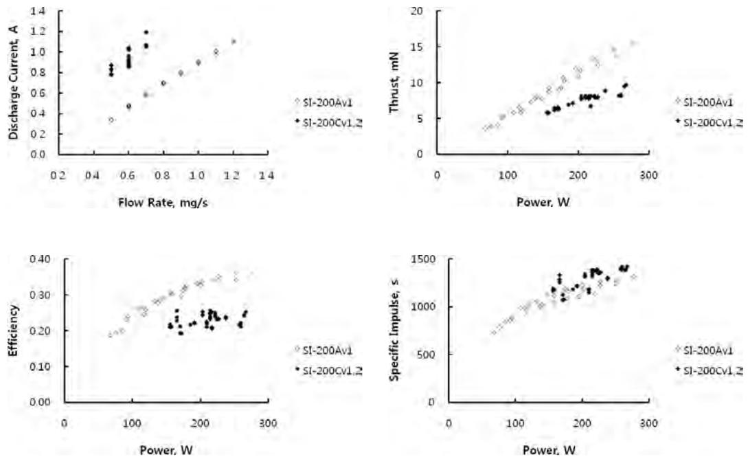
**Figure 5.** Performance comparison between the SI-200Av1 and the SI-200Cv-series in the voltage range of 200-250 V. Full markers denote the SI-200Cv-series and empty markers denote the SI-200Av1 thruster.
