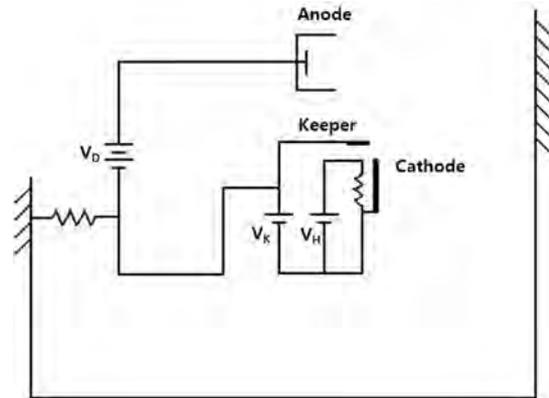
**Figure 3. Electric circuit diagram.  $V_D$  denotes the discharge voltage,  $V_K$  denotes the keeper voltage, and  $V_H$  denotes the heater voltage.**
