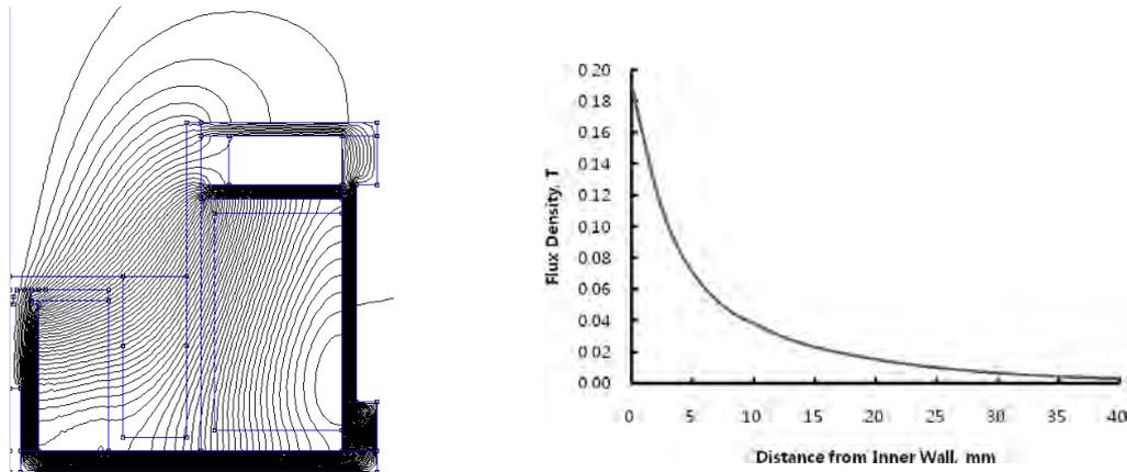
Figure 2. Sectional view of magnetic field structure and flux density curve at thruster axis.
