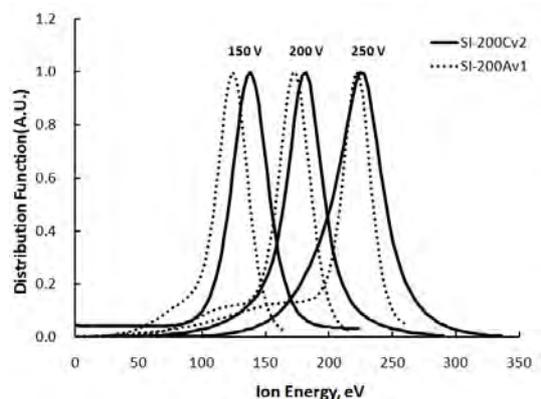
**Figure 8. Ion energy distribution for the SI-200Cv2 and the SI-200Av1 on the thruster axis at a mass flow rate of 0.6 mg/s**
