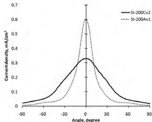
**Figure 7. Ion current density distributions for the SI-200Cv2 and the SI-200Av1 at 0.6 mg/s, 250 V.**
