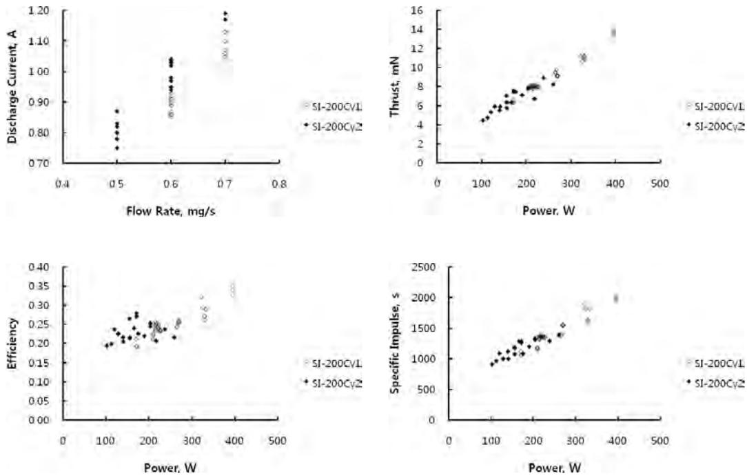
**Figure 4.** Performance comparison between the SI-200Cv1 in the voltage range of 200-350 V and the SI-200Cv2 in the voltage range of 125-250 V. Full markers denote the SI-200Cv2 and empty markers denote the SI-200Cv1 thruster.
