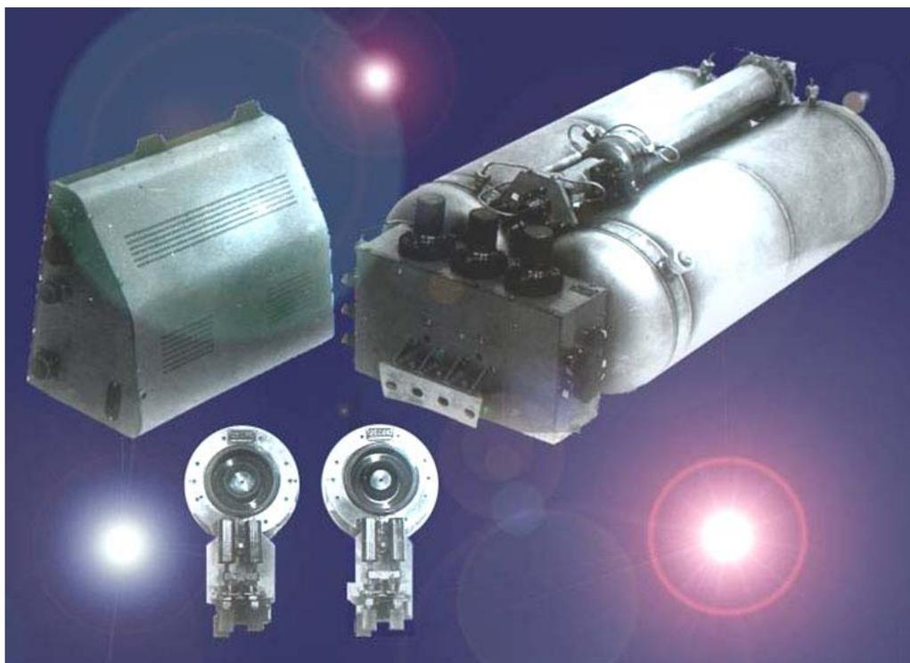
**Figure 9.** Parts of the 1<sup>st</sup> experimental propulsion system on base of SPT tested in 1972 on board of the Meteor satellite.
