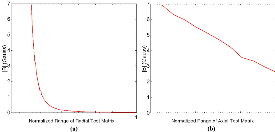
**Figure 8: Magnetic field decay in the radial (a) and axial (b) directions.** Graph (a) in the radial direction is for at the point of closest axial approach and graph (b) in the axial direction is for the point of closest radial approach. Both graphs follow the path of the external cathode from closest approach to farthest separation.
