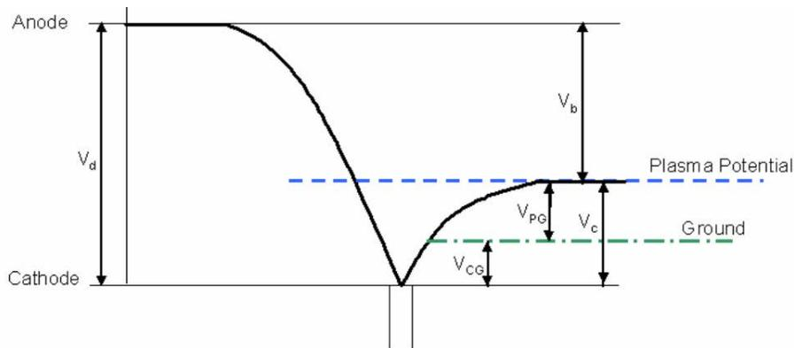
**Figure 1: Hall Thruster Conceptual Voltage Profile<sup>6</sup>**
