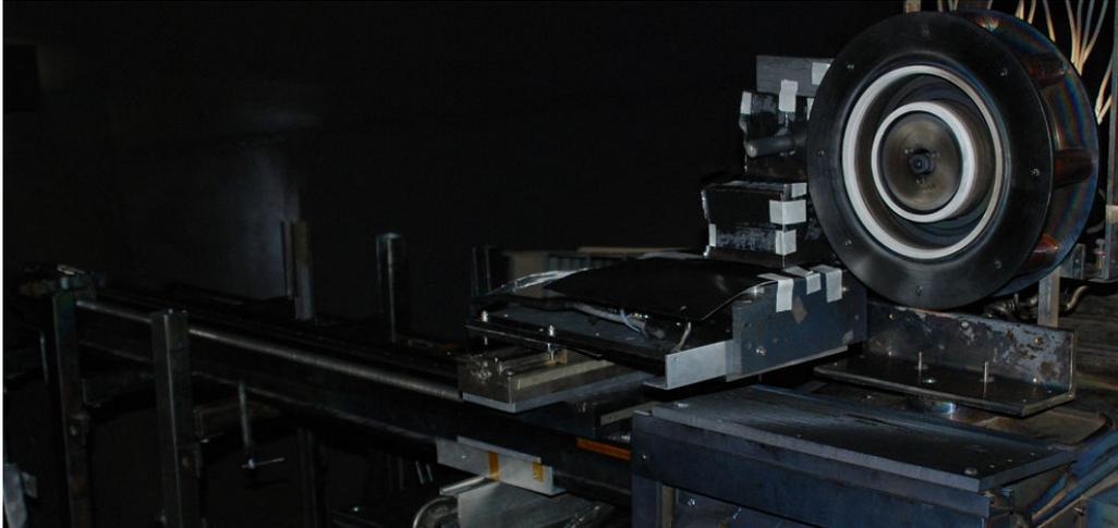
**Figure 6: External cathode axial, radial and theta motion system.** The external cathode is mounted on a 1.5 m radial table with a 30 cm axial table and a rotational stage. The rotational stage is hidden from view beneath graphite and Grafoil shielding.
