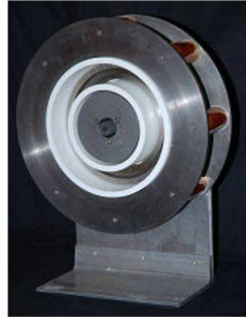
**Figure 2: The 6-kW laboratory model Hall thruster**
