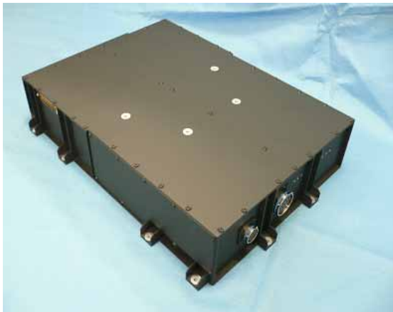
Figure 3. External view of EM2 PPU
