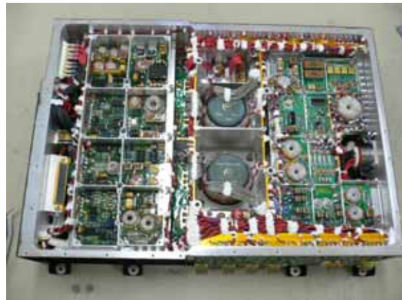
Figure 4. Internal view of EM2 PPU
