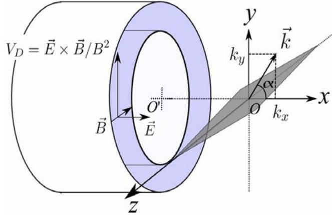
**Figure 2.** Scattering volume (dark gray) defined by the intersection of the primary and local oscillator beams. The inner plasma volume is in light gray. The coordinate system used has the radial magnetic field aligned with  $z$ , the axial electric field aligned with  $x$ , and the  $\vec{E} \times \vec{B}$  drift velocity,  $V_D$ , aligned with  $y$ .  $Ox$  is coincident with the thruster axis.
