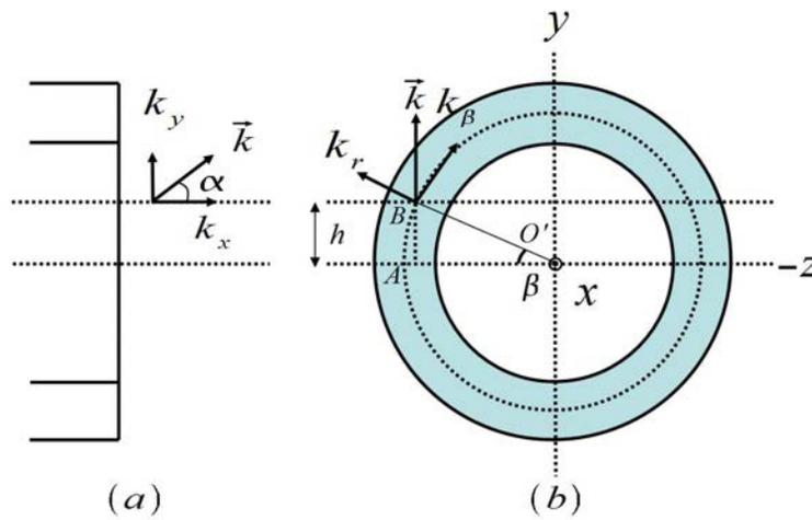
Figure 7. Positioning of measurement volume at different heights  $h$  with respect to thruster axis results in different values of  $k_r$ . (a) shows a side view of the thruster and  $k_x$  and  $k_y$  components; (b) shows the thruster face and  $k_r$  and  $k_\beta$  components.
