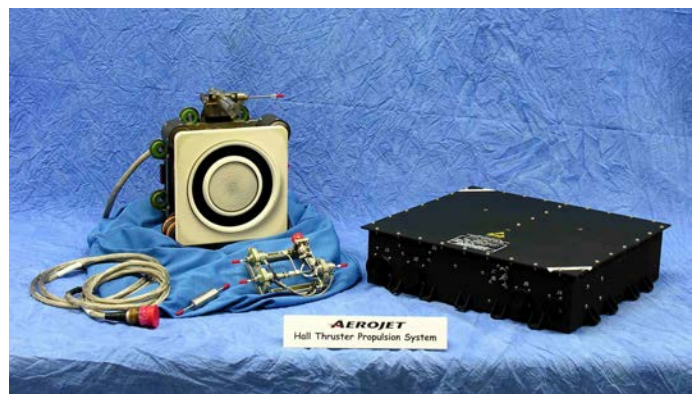
Figure 2. Hall thruster propulsion system- thruster, PPU, xenon flow rate controller, filter, and cable.
