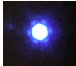
**Figure 11. Photograph of single-mode output beam from PCF.**
