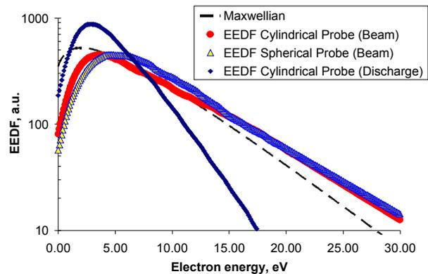
**Figure 4** Calculated simplified EEDF for a cylindrical and ellipsoid (near spherical) probe at 145 mN conditions. The ellipsoid EEDF is close to the centre of the grid. A Maxwellian distribution and EEDF obtained under 145 mN discharge conditions are also included.
