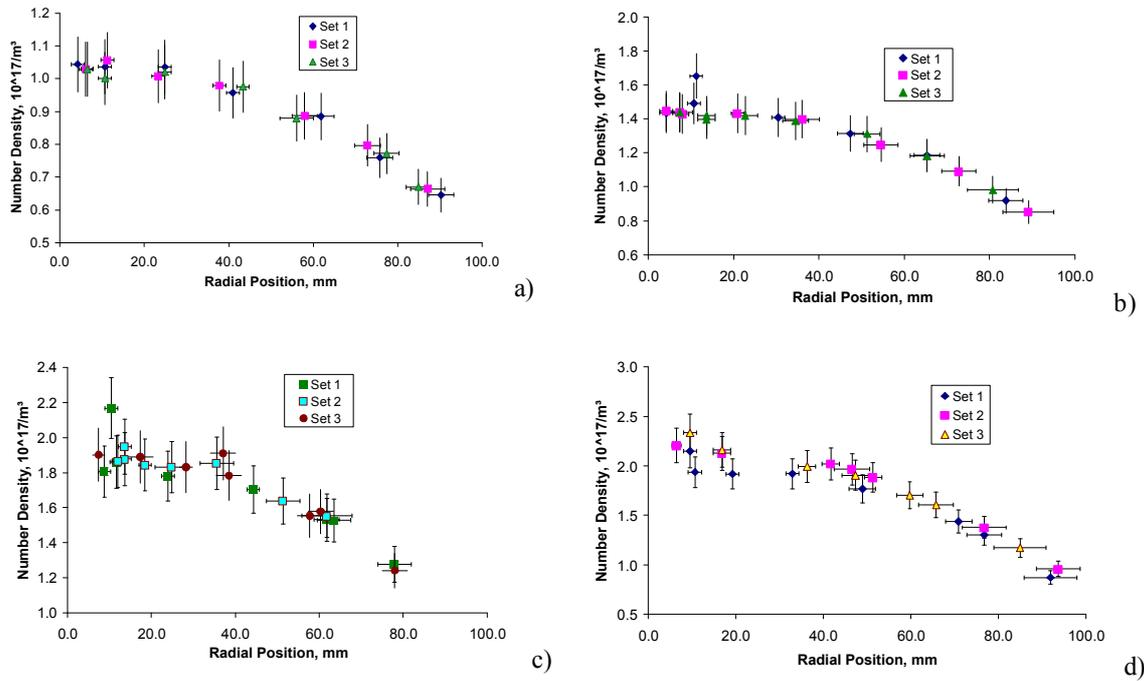
**Figure 5** Electron number densities, for thrust levels a) 75 mN b) 100 mN c) 125 mN and d) 145 mN, calculated using the Druyvesteyn method and assuming an ellipsoid geometry as measured afterward.
