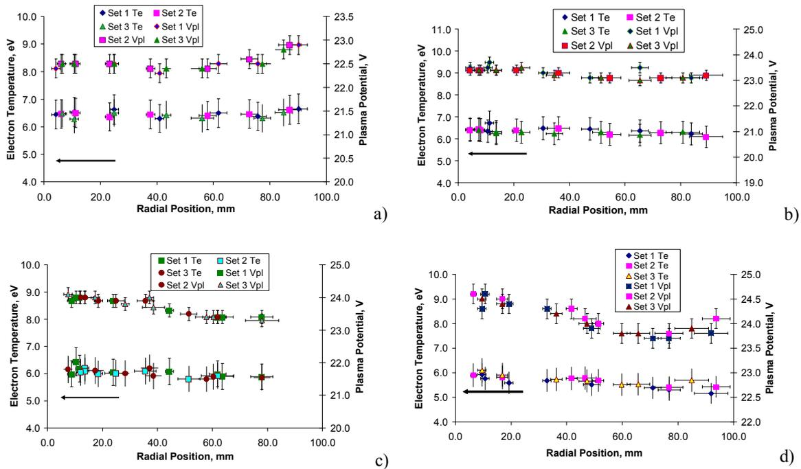
**Figure 5** Electron temperatures and plasma potentials, for thrust levels a) 75 mN b) 100 mN c) 125 mN and d) 145 mN, calculated using the Druyvesteyn method and assuming an ellipsoid geometry as measured afterward.
