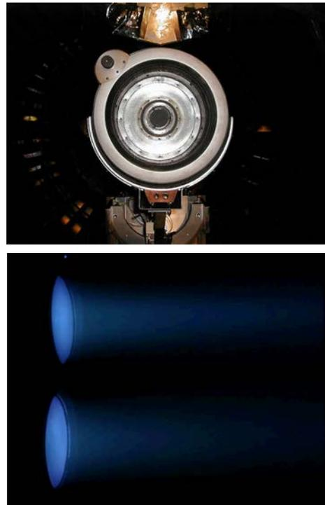
**Figure.1 A typical T6 thruster (left) and simultaneous operation of two thrusters (right).**
