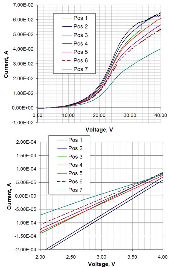
**Figure 3 LP traces taken at 145 mN operating conditions. Top shows the traces in their entirety; Bottom shows the floating potential which reduces with increasing radial position.**
