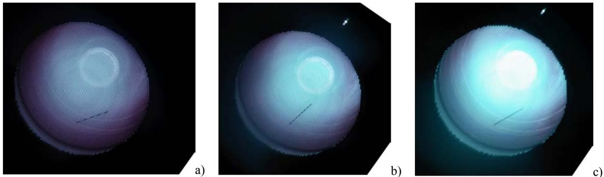
**Figure 2. Photographs of the T6 thruster firing during LP testing showing the probe in different positions. The photographs were taken at the following thrust levels a) 75 mN, b) 100 mN and c) 145 mN.**
