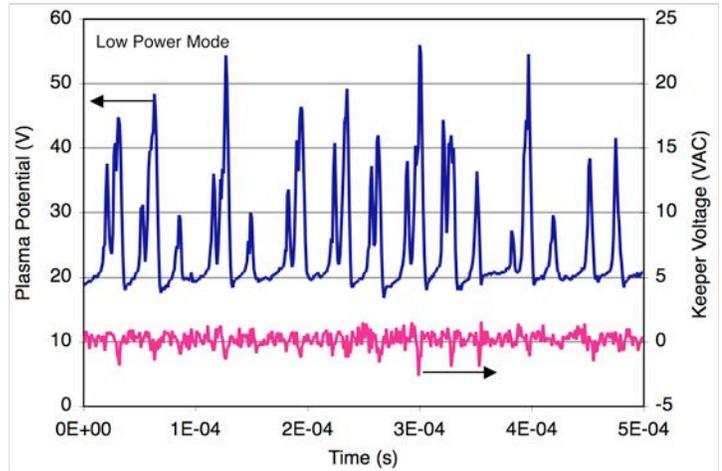
**Figure 8. Plasma potential in the cathode plume and AC keeper voltage in the low power mode of the NCA discharge showing large oscillation levels.**
