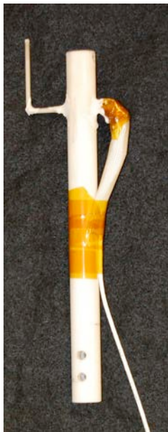
Figure 3: Translatable Langmuir probe and macor extension arm
