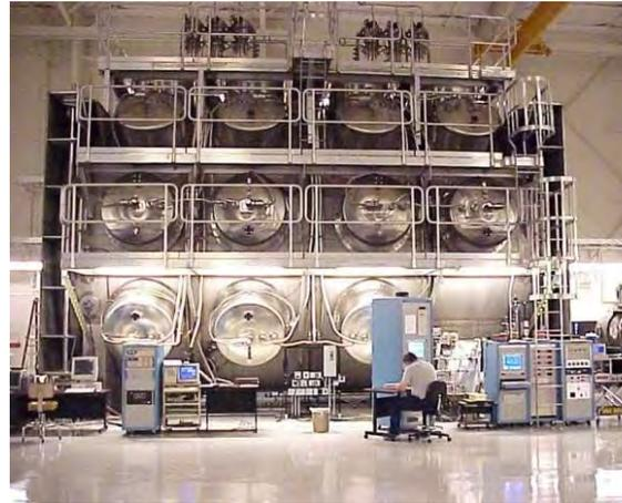
Figure 3. Life Test Chamber used for the Q2, 25 cm XIPS<sup>®</sup> Thruster at L-3 ETI.
