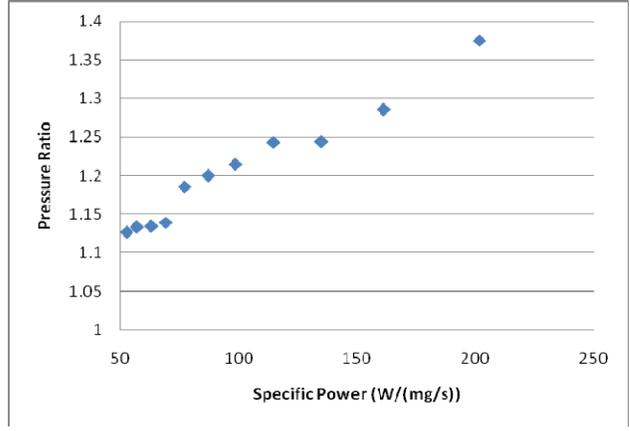
Figure 13. Specific power vs. pressure ratio.
