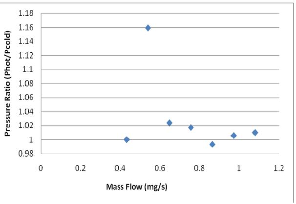
**Figure 4a. Pressure ratio vs. mass flow for experiment 1.**
