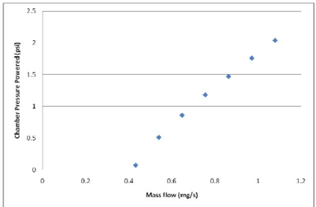
**Figure 4b. Chamber pressure (powered) vs. cold flow experiment 1.**
