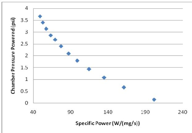
Figure 14. Specific power vs. powered chamber pressure.
