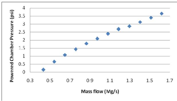
Figure 10. Powered mass flow vs. chamber pressure.
