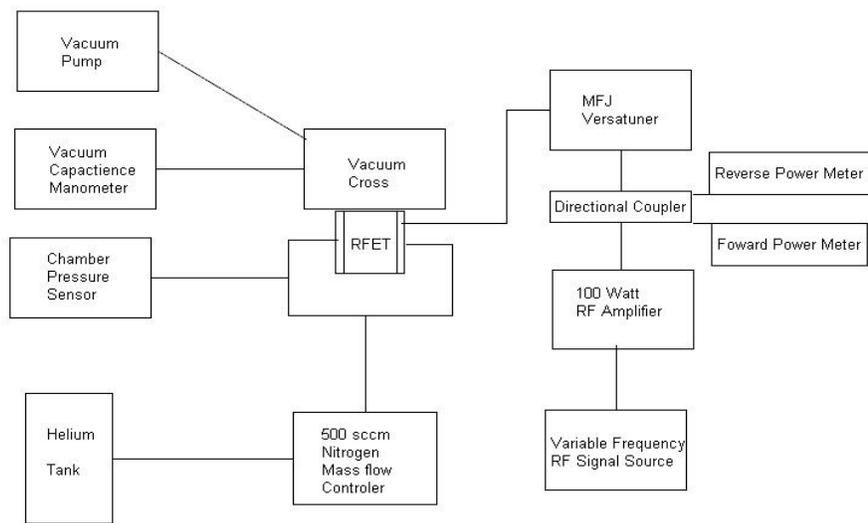
**Figure 2. Experimental setup 1.**
