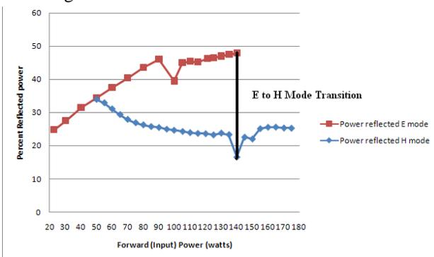
**Figure 8. Percent reflected vs. input power.**
