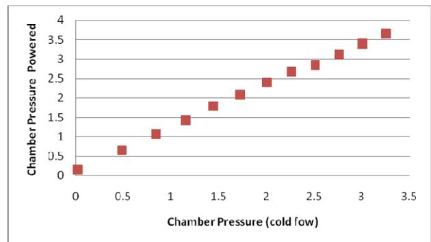
Figure 11. Cold flow pressure vs. powered pressure.
