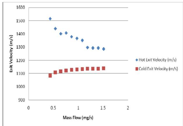
Figure 15. Mass flow vs. hot and cold calculated exit velocities.
