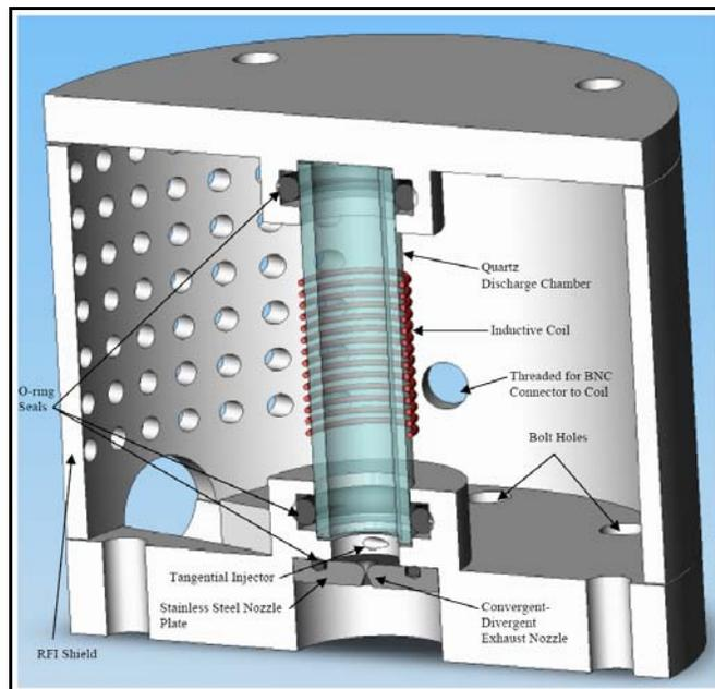
Figure 1. Diagram of RFET design.
