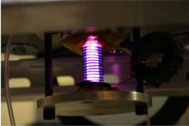
**Figure 16. Powered H-mode operation showing anomalies at the top and bottom of the quartz chamber.**
