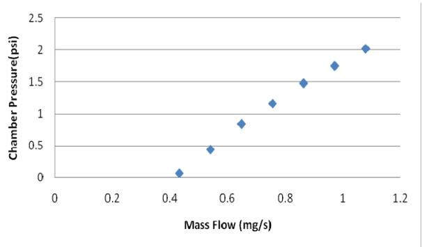
**Figure 3. Cold flow pressure data for experiment 1.**
