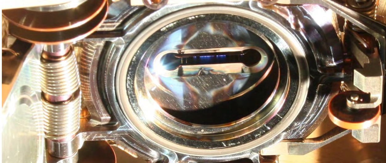
Figure 7. Thruster firing in IV1 facility @ 150 \mu N thrust (Priming Test No. 2 / Endurance Test No. 2).
