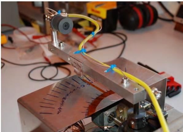
**Figure 3. Rotatable beam probe assembly with gridded faraday cup.**
