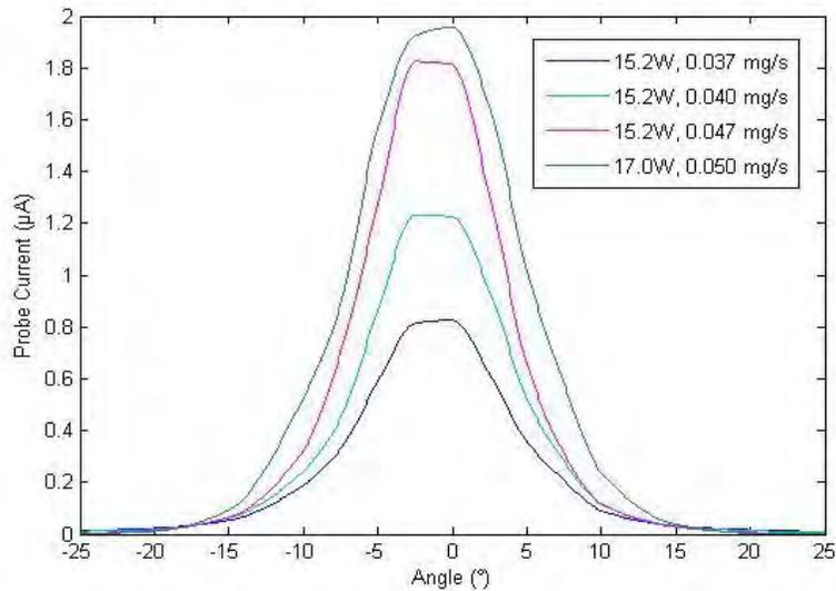
**Figure 12. Radial beam profiles for SE1 for different thrust levels.**
