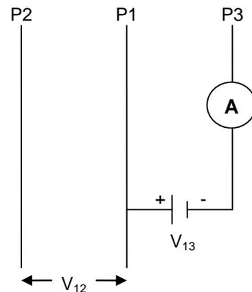
**Figure 4. Triple Langmuir probe circuit for direct-display of electron temperature and density.**
