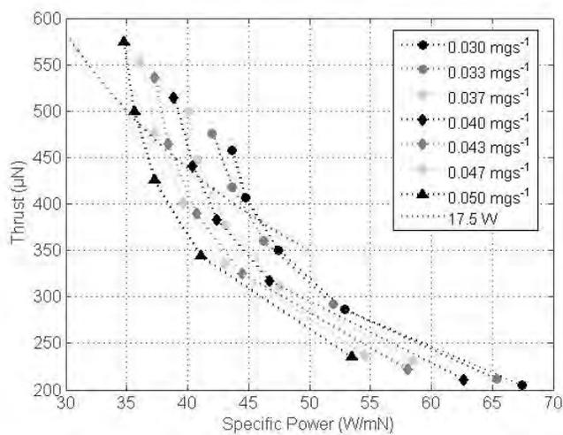
**Figure 9. Estimated thrust against specific power for the SE2 configuration.**
