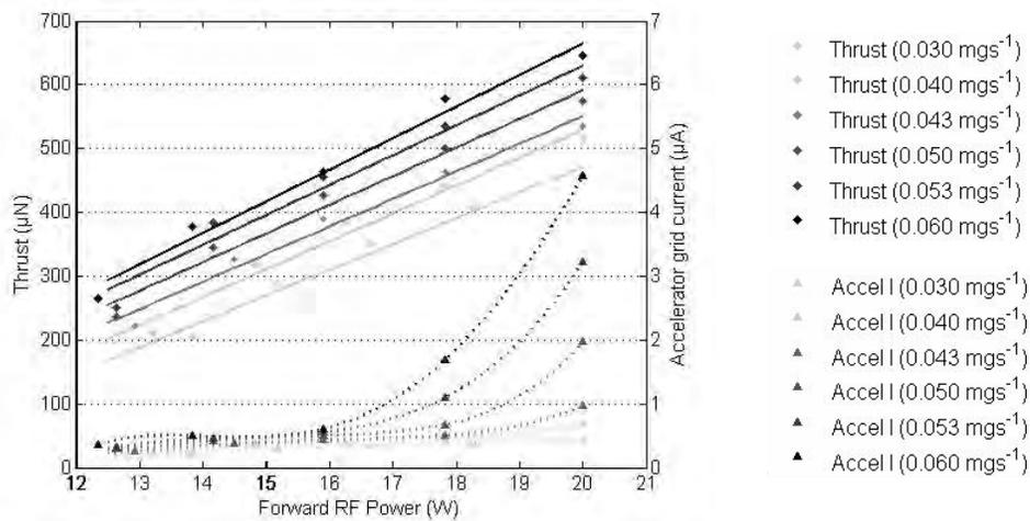
**Figure 8. Estimated thrust and measured accelerator grid current for different RF power and flow rates for the SE2 configuration.**
