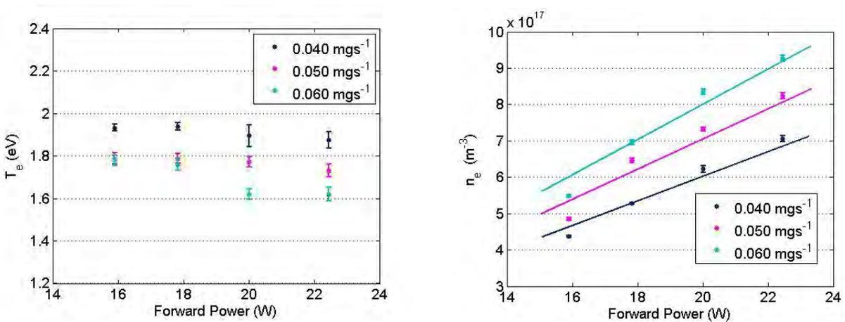
**Figure 13. Estimated electron temperature and density for different RF power and flow rates.**
