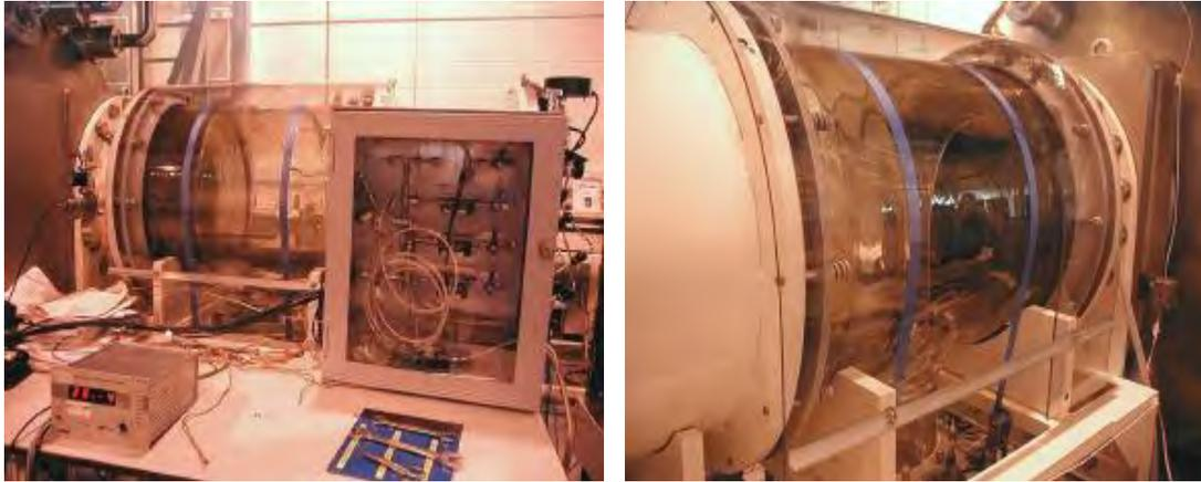
**Figure 2. Loadlock chamber of LEEP-1 facility.**
