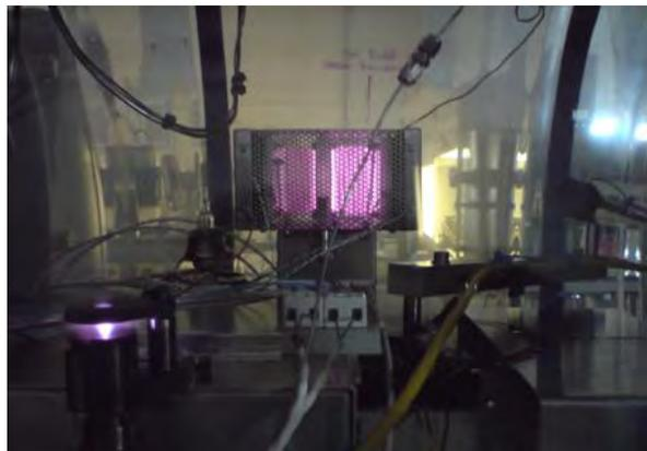
**Figure 7. The MiDGIT breadboard thruster operating in single-ended mode with a hollow cathode neutraliser.**
