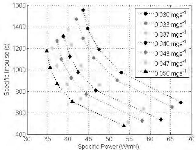
**Figure 10. Specific impulse against specific power for the SE2 configuration.**
