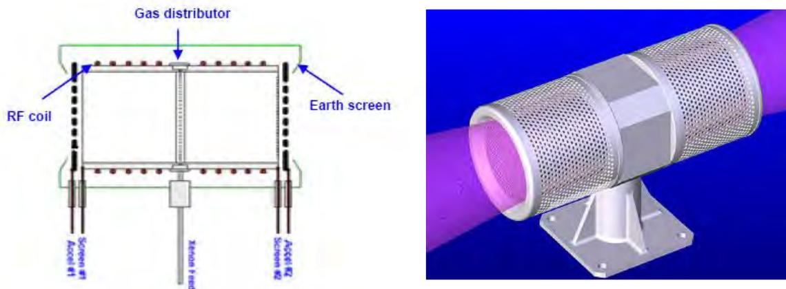
Figure 1. The basic configuration of the MiDGIT Thruster
