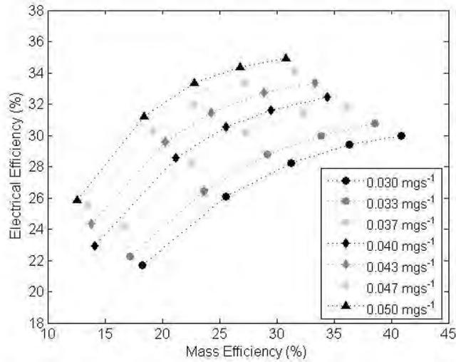
**Figure 11. Electrical efficiency against mass utilization efficiency for the SE2 configuration (neglecting neutraliser power and flow rate).**
