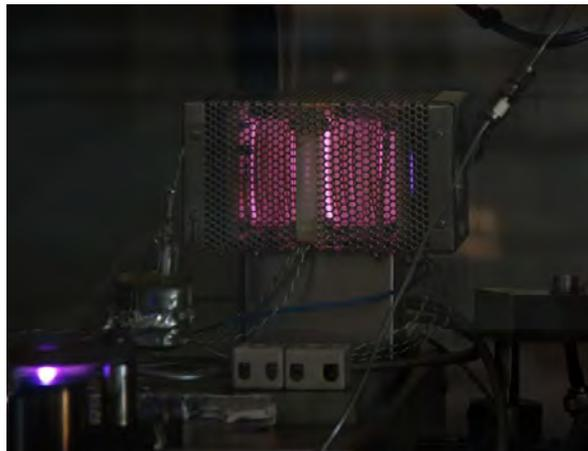
**Figure 14. The MiDGIT breadboard thruster operating in differential mode with a hollow cathode neutraliser.**
