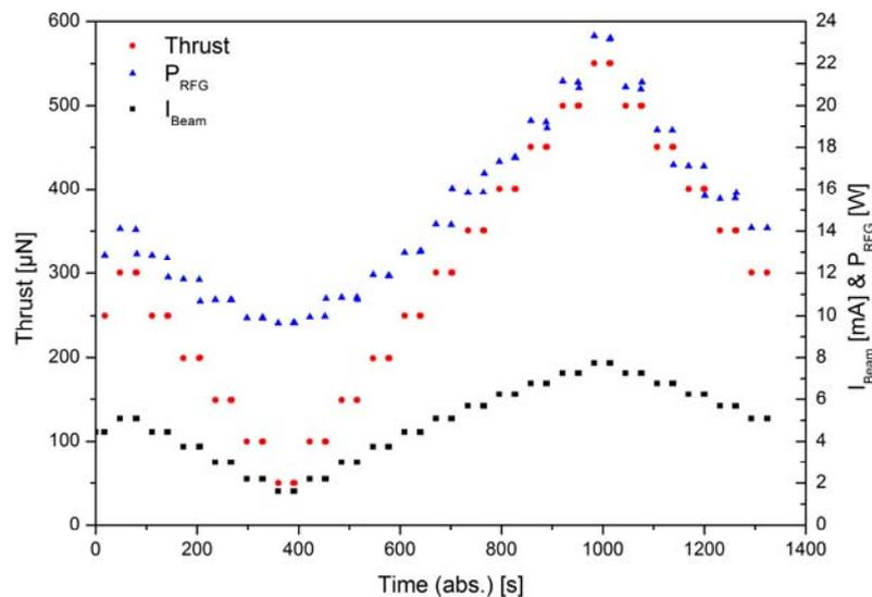
**Fig.6: Thrust stepping experiment of  $\mu\text{NRIT-2.5}$**
