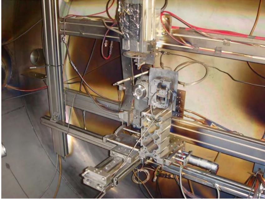
Fig. 2: Microthruster  $\mu$ NRIT-2.5 installed on a test platform in the facility “Big Mac”.<sup>7,10</sup>
