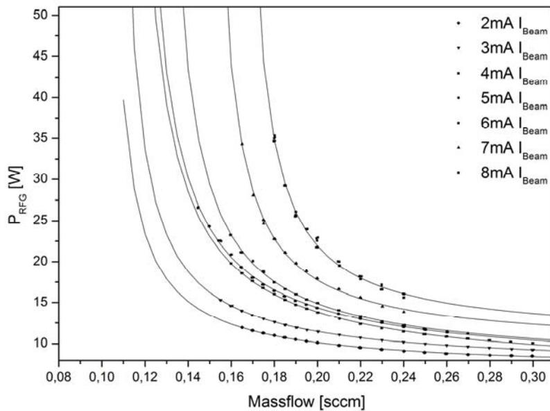
Fig. 3: Extracted beam current (2mA to 8mA as the parameter) of  $\mu$ NRIT-2.5 as function of the required rf-generator power  $P_{\text{REG}}$  and the propellant flow rate MFC.<sup>7,10</sup>
