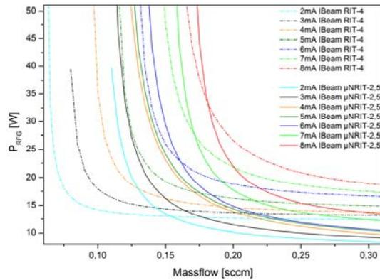
**Fig. 4: Comparison of the discharge characteristics IBeam ( $P_{REG}, \dot{V}$ ) of the Giessen  $\mu$ NRIT-2.5 engine<sup>7, 10</sup> and of the 4cm microthruster RIT- $\mu$ x of EADS-Astrium;<sup>4</sup> both engines are equipped with a two-grid system having 37 beamlet borings.**
