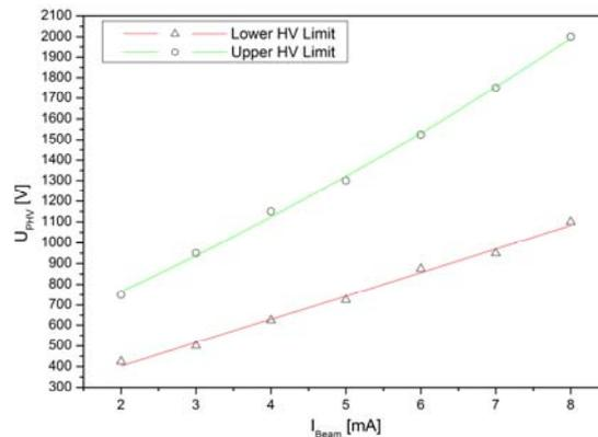
**Fig. 5: Range of the positive high voltage  $U_{PHV}$  (with upper and lower borders) in which the optimum focusing of the beamlets are maintained vs. the beam current  $I_{Beam}$ .<sup>7, 10</sup>**
