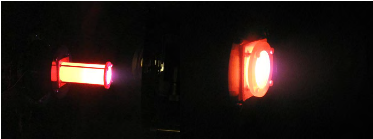
Figure 22 T6VLA operating at 25A, 0.1mg/s (left) T6 SA operating at 12.5A, 0.1mg/s (right)
