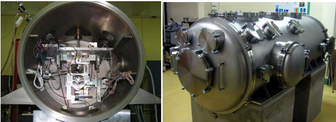
Figure 5. Small vacuum tank and balance mounted (left) and new B09 facility (right).
