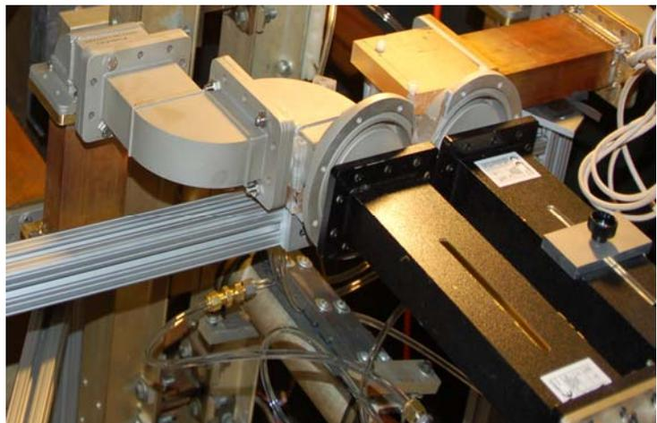
**Figure 6. View of the close range antennae on the thrust stand.** *The clear colored close range antenna is distinguished by its deep groove and circular rim. The distance between the thruster feed and the antenna is comprised between 10 and 30 mm.*
