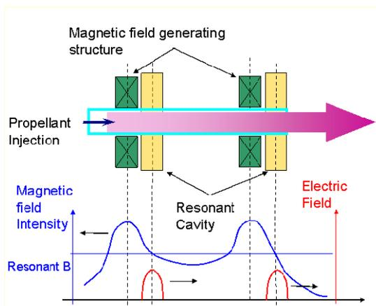
**Figure 1. Overview of the basic structure of the electrodeless thruster.** The magnetic structure creates an axial magnetic field featuring a magnetic bottle and a diverging field suitable for ponderomotive force acceleration.
