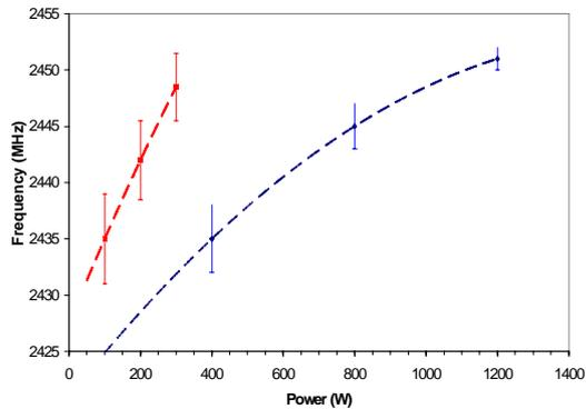
**Figure 6. Microwave generators frequency variation requested power output.** *The frequency accuracy of the generators are excellent for a given power output. However, the spectrum shift and reach the nominal frequency at the nominal power output of each generator.*
