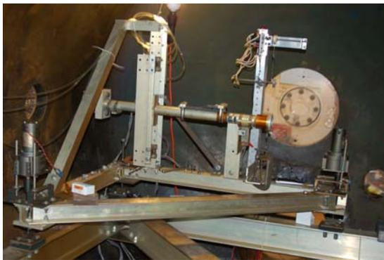
**Figure 4. LDPP thrust stand.** The horizontal arm rotate around the vertical axis on the left side of the picture. The motor at the lower left corner and on the right side of the picture allow adjusting the orientation of the thrust stand axis. Behind the arm the vertical support of the thrust calibration system is visible
