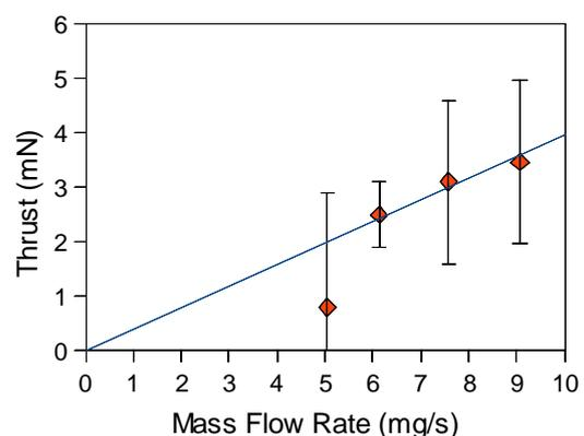
**Figure 5. Cold thrust measurements at various argon mass flow rate.** The thrust measured by the thrust stand is represented by the red data points along with their uncertainty. The blue line represents the cold thrust calculated from theory.
