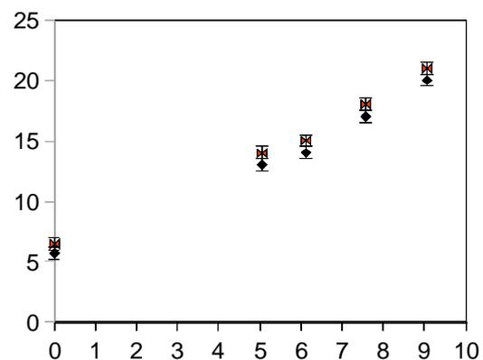
**Figure 3. Steady state pressure in SSLP at various mass flow rate.** The pressure is displayed in  $10^{-5}$  Torr unit and the mass flow rate in mg/s Red and black mark display the small but measurable difference between the pressure at the end of the vacuum chamber and at the pump inlet.
