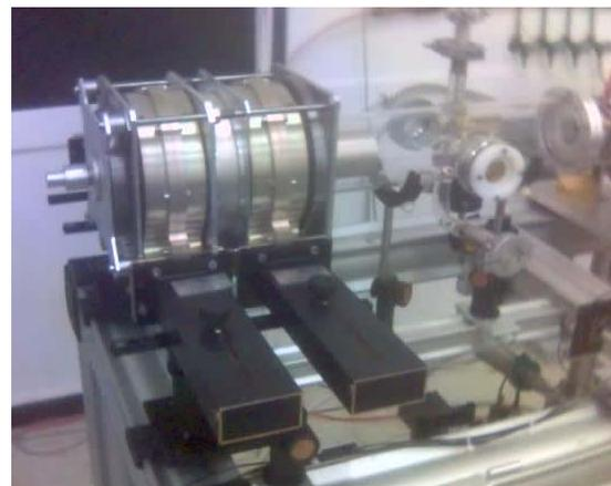
**Figure 2. The High Power Electrodeless Plasma Thruster on test bench at ONERA.** Each resonator (golden cylinders) is attached to one of the microwave tuning element (black rectangles in front). The thruster is producing a plasma beam in the small glass vacuum vessel at the right.
