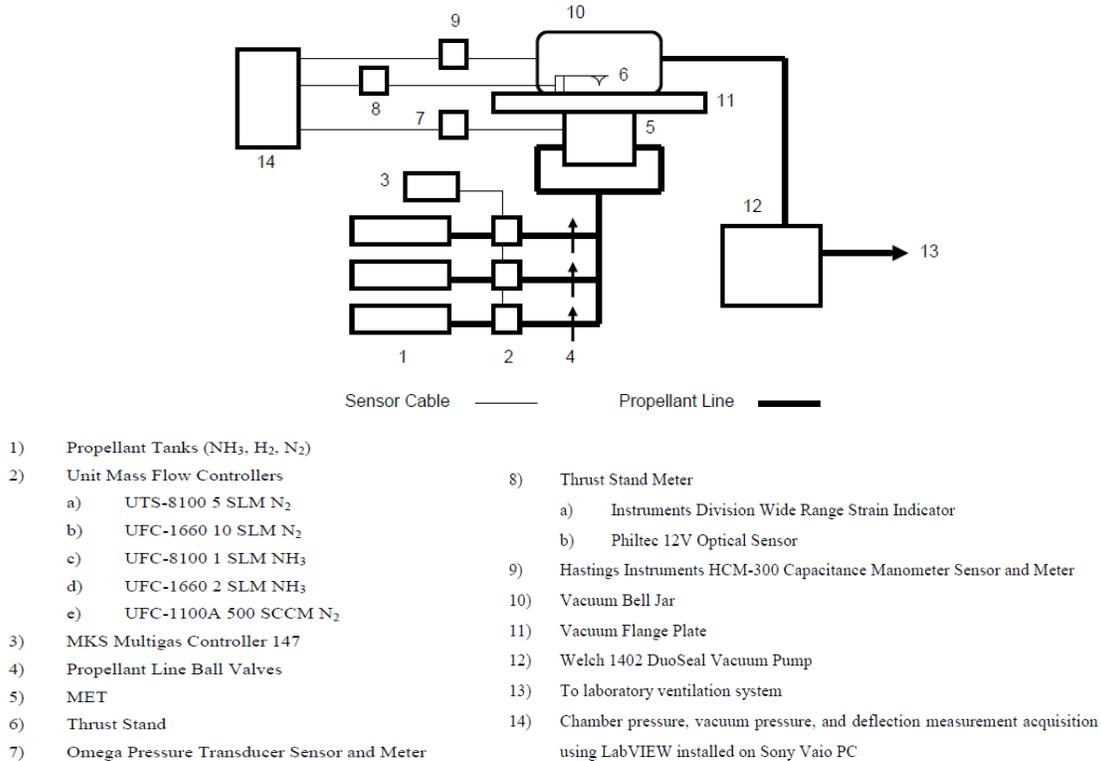
**Figure 2. MET propellant control system.**
