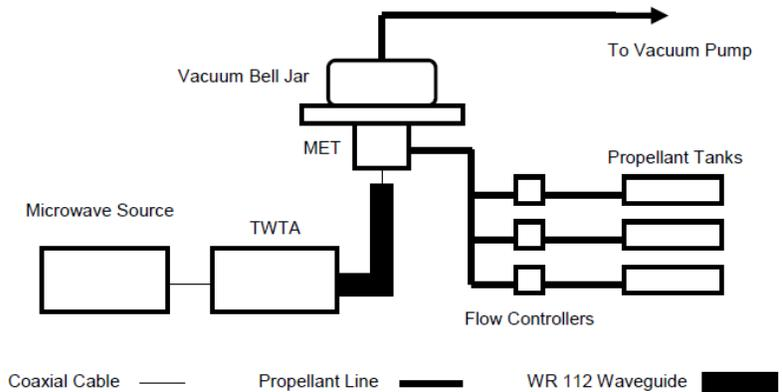
Figure 1. Overall schematic of MET test apparatus.
