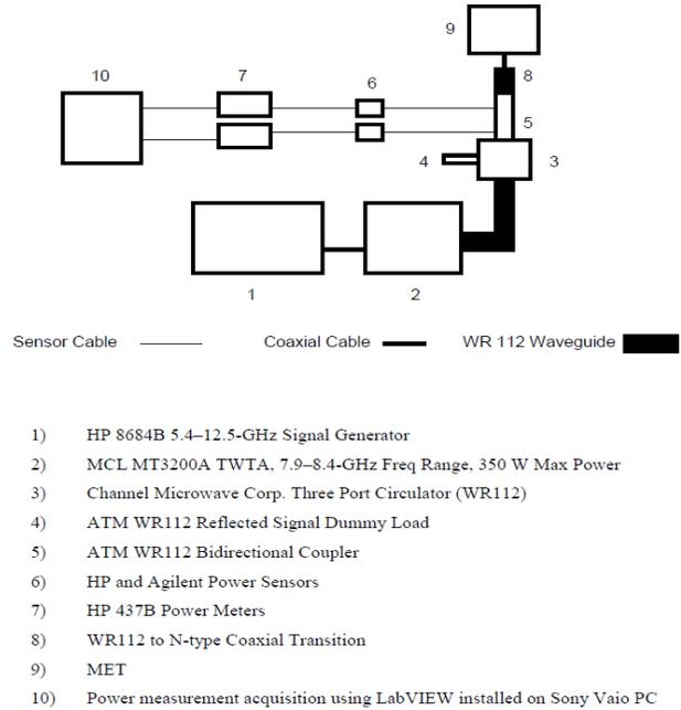
Figure 3. Electromagnetic control system.
