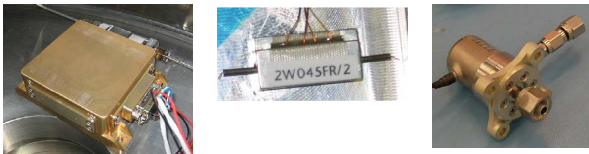
Figure 6: Micro flow sensor and sensing element (mass: 419 g, envelope 37 x 113 x 120 mm) and proportional flow control valve (mass: 175 g, envelope 31 x 51 mm) on the left.
