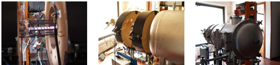
Figure 1. Current CISAS experimental set-up with Helmholtz-magnetic-coils.
