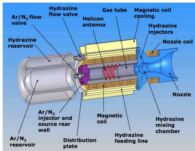
Figure 1. Schematics of the HPH.com helicon thruster.
