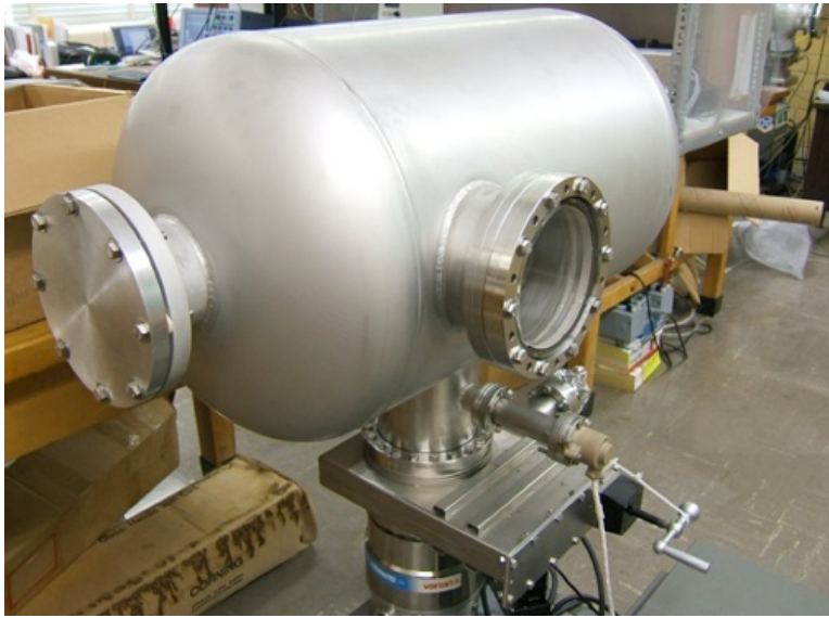
Figure 3. MadHeX Expansion Chamber, not installed in system.
