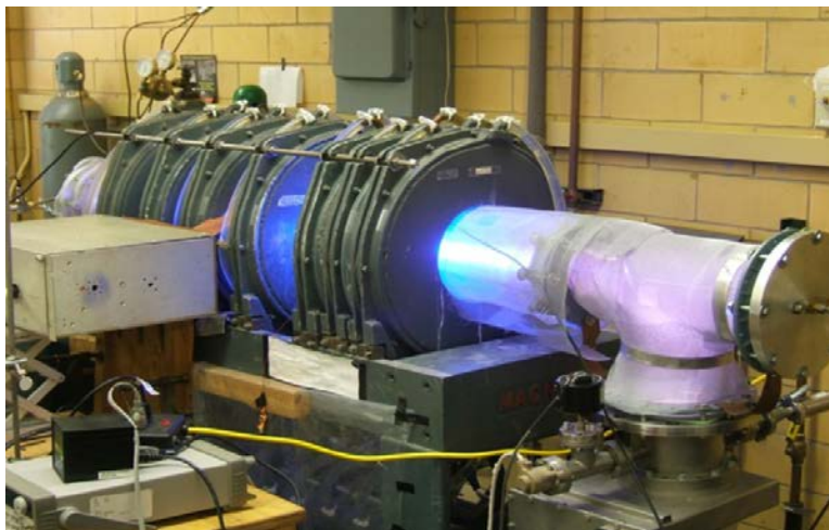
Figure 2. Operation of MadHEX at 3 kW input power.
