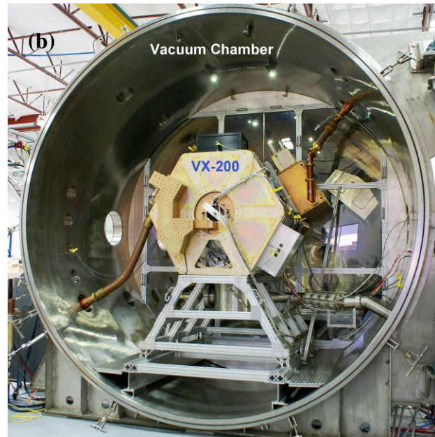
Figure 2. a) Image of a simplified 3-d model of the VX-200 with a point of view from the aft end. b) Photograph of the VX-200 installed in the large chamber at Ad Astra Rocket Company.
