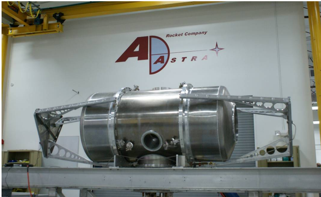
Figure 4. Photograph of the low temperature superconducting magnet with alignment fixtures mounted to the ends.
