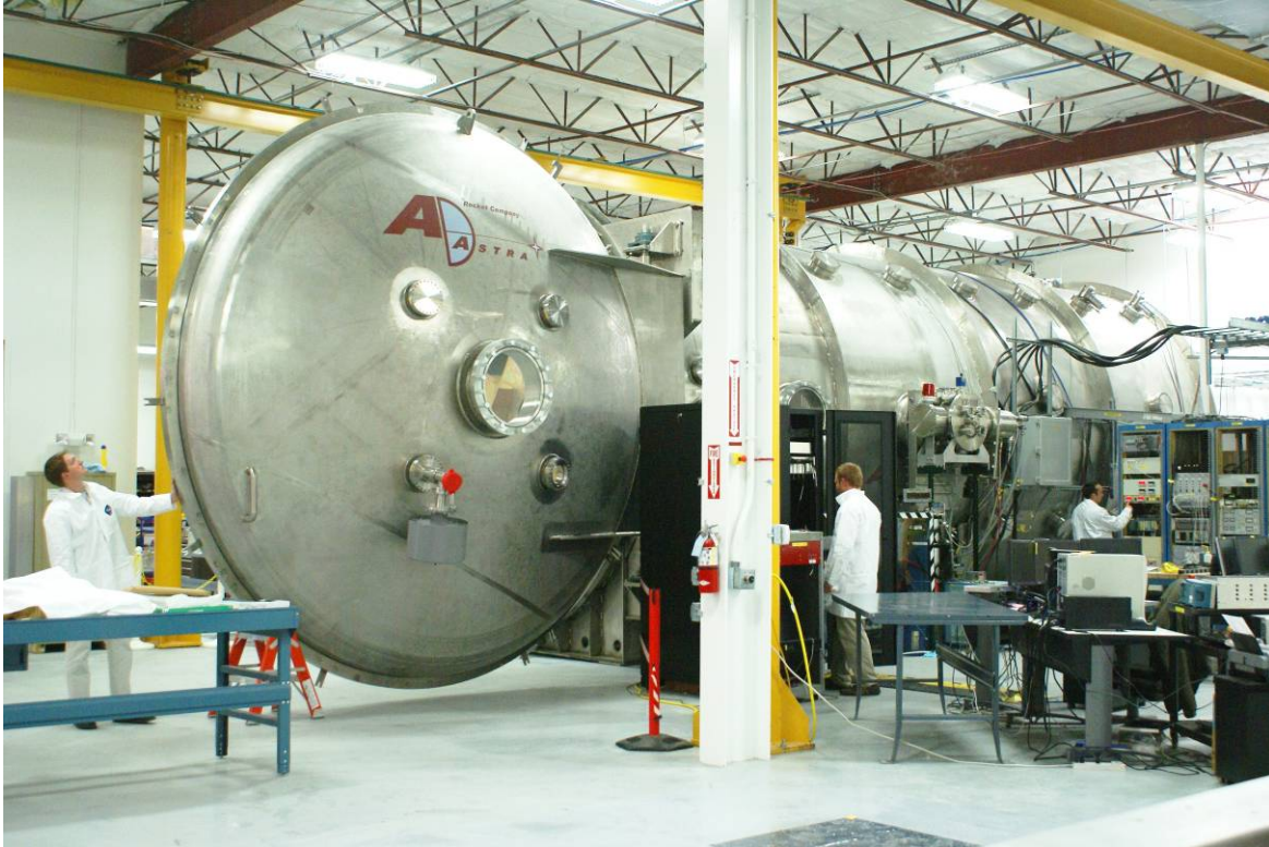
Figure 5. Photograph of the “El Monstruo” large vacuum chamber at Ad Astra Rocket Company.
