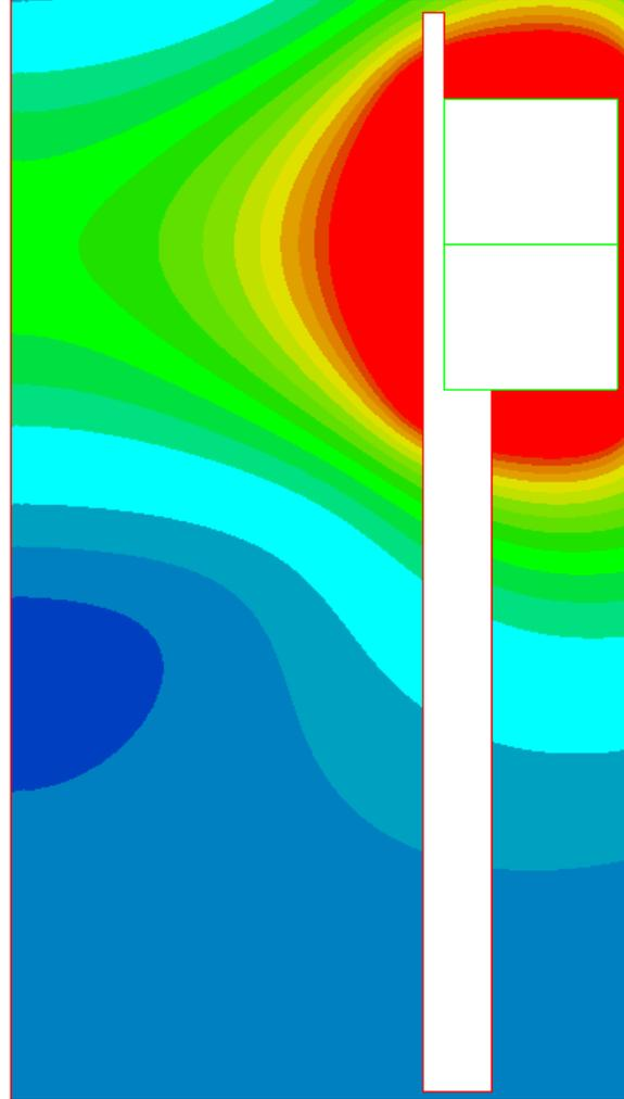
**Figure 1. Contour plot of magnetic field strength within waveguide. Leftmost edge is waveguide axis. ECR heating zone shown in bright green.**
