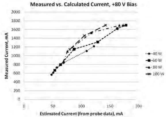
**Figure 16. Measured current vs. expected current from Langmuir data.**
