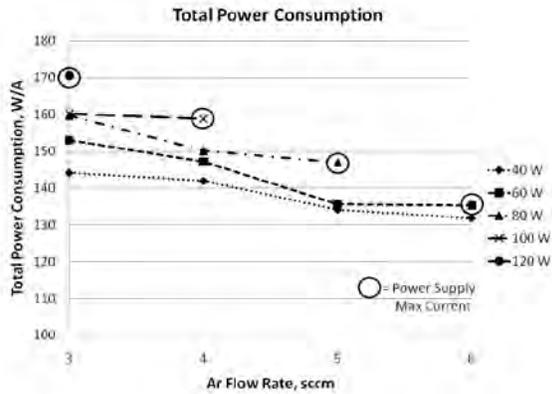
Figure 12. Total power consumed per Ampere. 4 mm extraction orifice, and 100 V bias.
