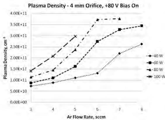
Figure 14. Plasma density from Langmuir probe traces. 4 mm extraction orifice, and 80 V bias.
