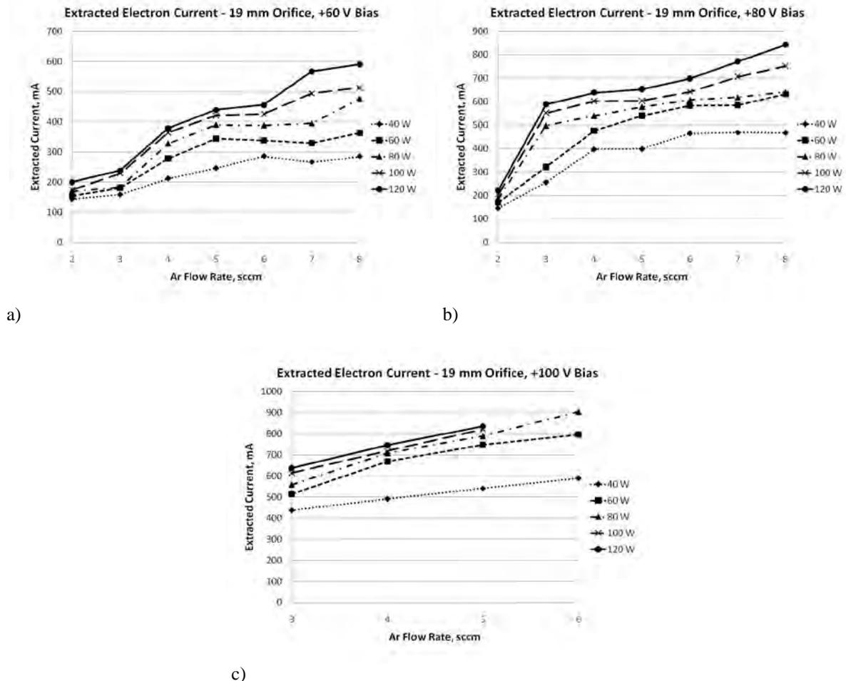
**Figure 7. Extracted electron currents versus microwave power and flow rate, for 19 mm extraction orifice, and electrode bias of: a) 60 V, b) 80 V, and c) 100 V.**
