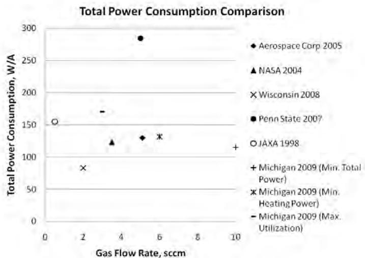
**Figure 18. Total power consumption versus flow rate, for several plasma cathodes in the literature.**
