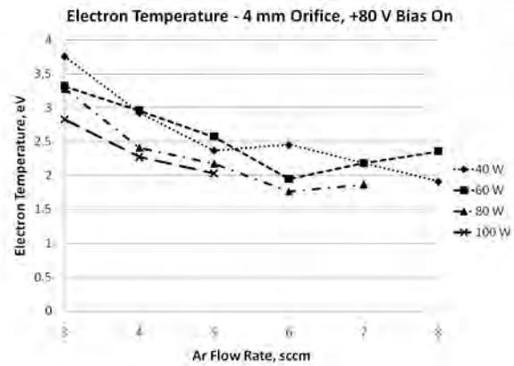
Figure 15. Electron temperature from Langmuir probe traces. 4 mm extraction orifice, 80 V bias.
