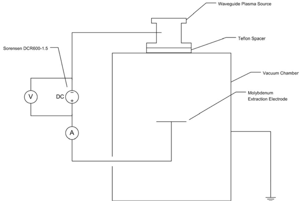
Figure 5. Schematic of electron current extraction circuit.
