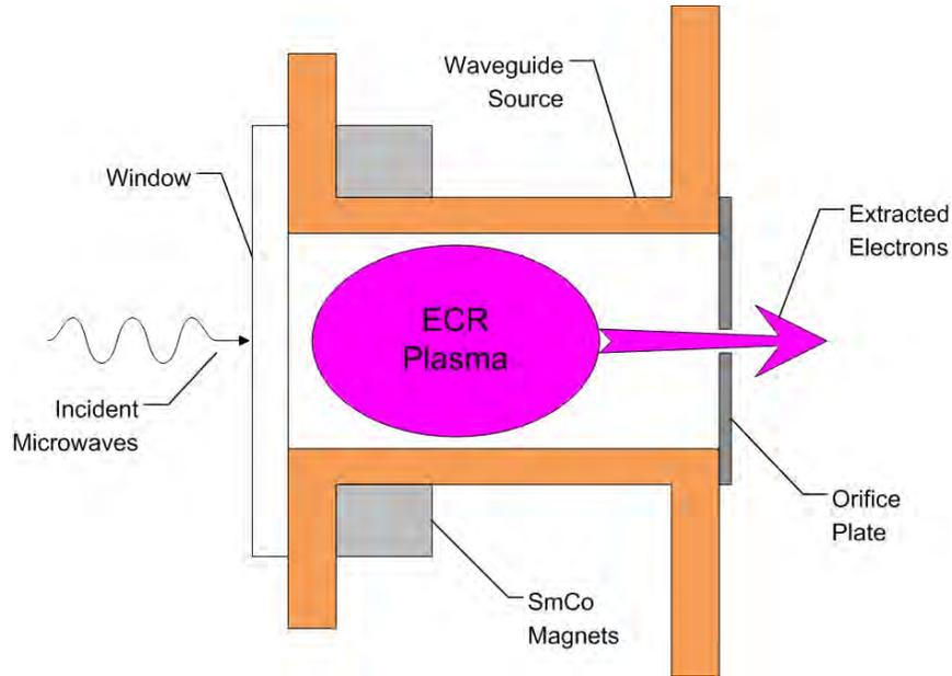
**Figure 2. Sketch of the waveguide plasma cathode.**
