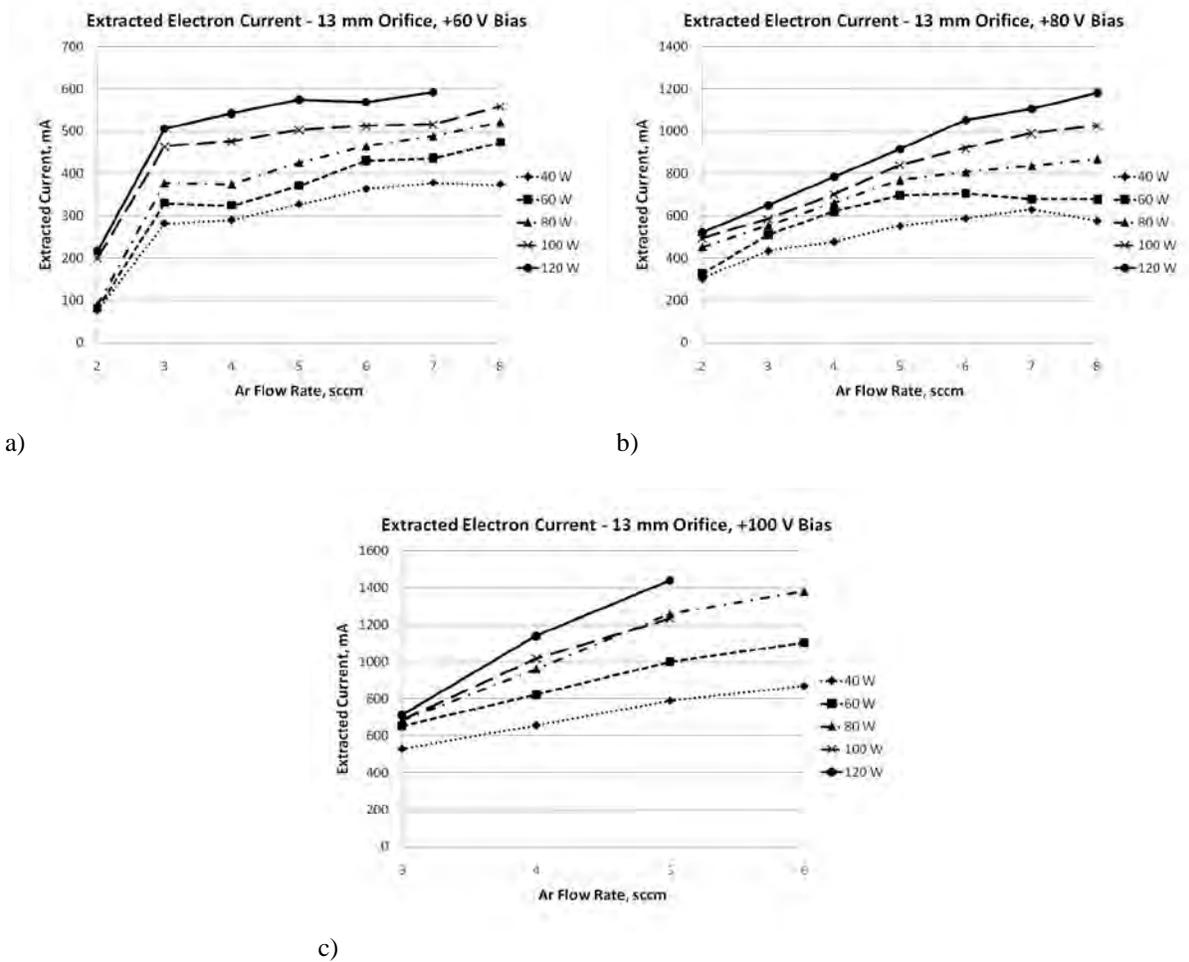
**Figure 8. Extracted electron currents versus microwave power and flow rate, for 13 mm extraction orifice, and electrode bias of: a) 60 V, b) 80 V, and c) 100 V.**
