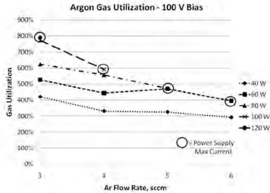
Figure 13. Feed gas utilization. 4 mm extraction orifice, and 100 V bias.
