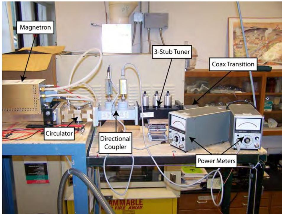
**Figure 4. Photograph of the microwave setup.**
