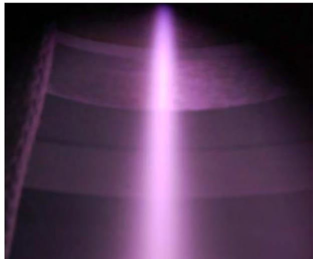
**Figure 10. Plasma plume emanating from the extraction orifice of the plasma source (top).**
