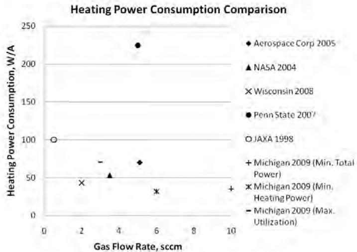
**Figure 17. Heating power consumption versus flow rate, for several plasma cathodes in the literature.**
