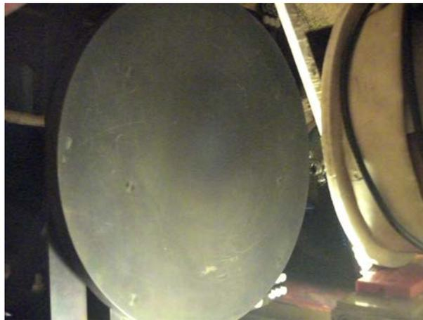
Figure 16. The Target's Plate after several Mira C firings: radial shading is due to plasma impact burns. The electromagnet can be seen on the right side.
