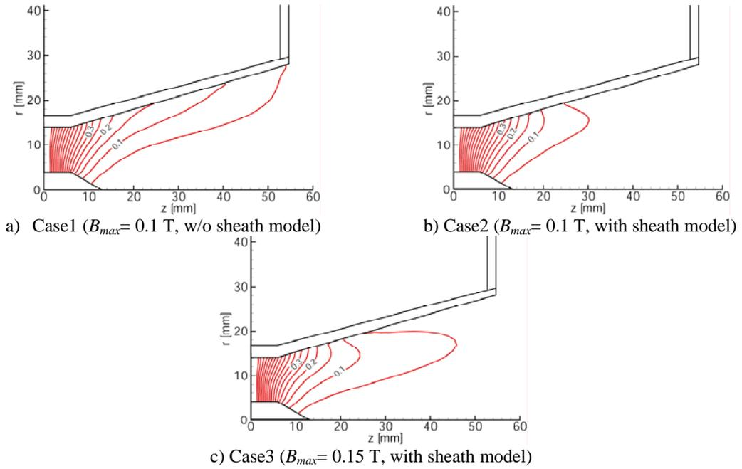
**Figure 4.** Current contour lines, Ar, 0.1 g/s,  $J = 1$  kA.
