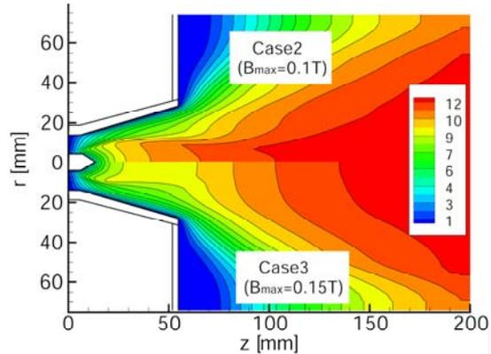
Figure 8. Axial velocity distribution, km/s, Ar, 0.1g/s,  $J = 1$  kA.
