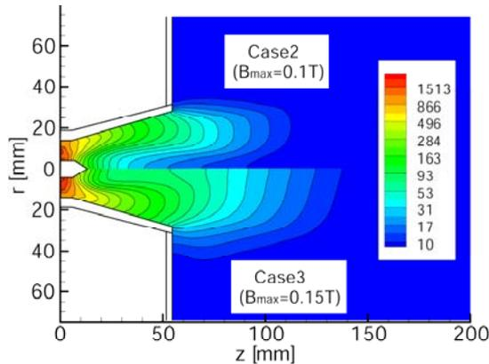
Figure 10. Pressure distribution, Pa, Ar, 0.1g/s,  $J = 1$  kA.
