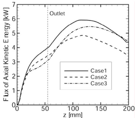
Figure 7. Energy flux of axial kinetic energy, Ar, 0.1g/s,  $J = 1$  kA.
