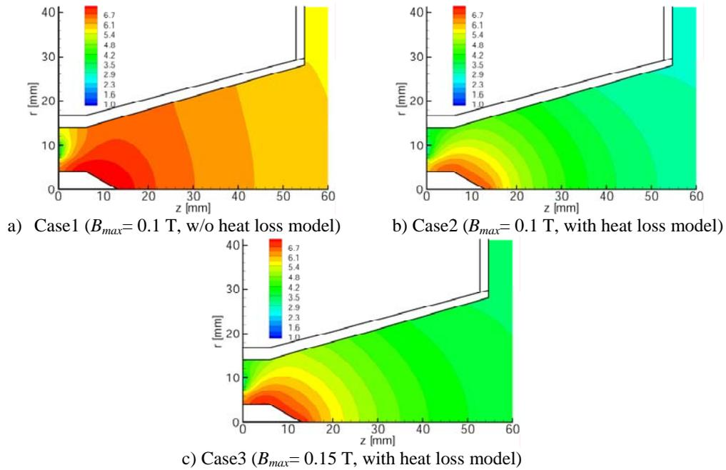
**Figure 6. Electron temperature, eV, Ar, 0.1 g/s,  $J = 1$  kA.**
