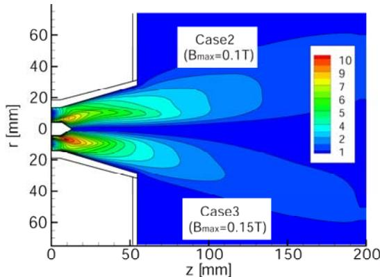
Figure 9. Azimuthal velocity distribution (absolute value), km/s, Ar, 0.1g/s,  $J = 1$  kA.
