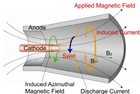
Figure 1. Principle of applied-field MPD thruster.
