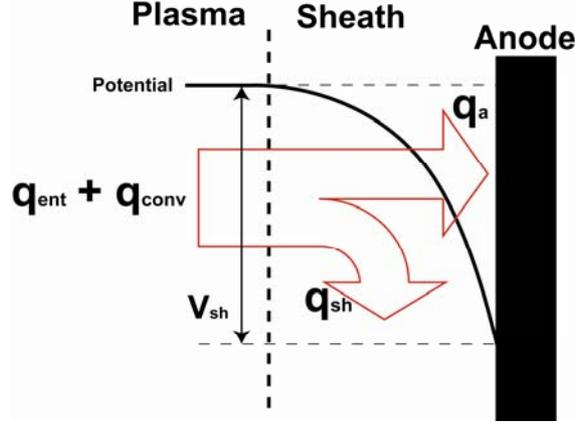
**Figure 3. Electron energy balance on anode (An ion-rich sheath is assumed. The sheath voltage  $V_{sh}$  is defined so as to be a positive value.).**
