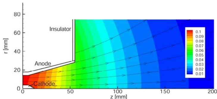
Figure 2. Thruster geometry and distribution of applied magnetic field, T, ( $J_c = 10$  A).
