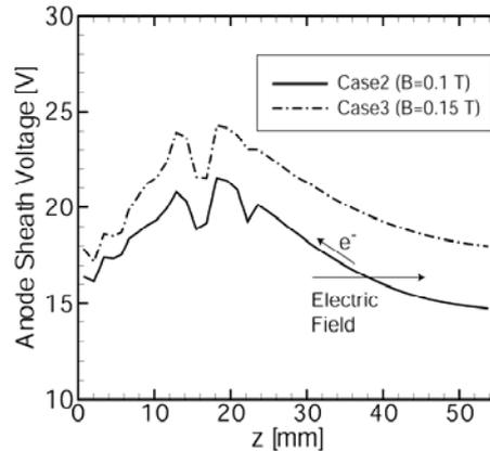
**Figure 5.** Anode sheath voltage along the anode surface (An ion-rich sheath is assumed. The sheath voltage  $V_{sh}$  is defined so as to be a positive value.).
