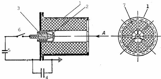
**Figure 4. Electrothermal APPT: 1,2 electrodes; 3- carborundum, 4- primary discharge capacitor bank, 5- discharge initiation capacitor, 6 -switch, 7 - propellant.**
