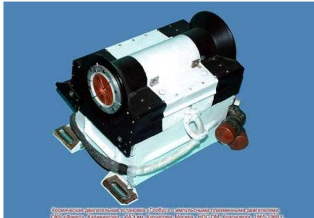
Figure 7. Space propulsion system “Globus” with pulsed plasma thrusters produced by the Experimental Design Bureau “Fakel”, Kaliningrad – Kurchatov Institute of Atomic Energy, Moscow – NPO PM, Krasnoyarsk
