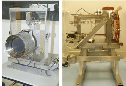
Figure 4. a) 1-axis optical thrust stand with GIS-15 and b) Low thrust balance
